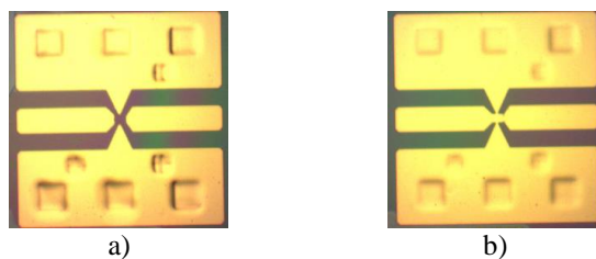
Fig. 1. G0 test structures' layout: a) transistor's open; b) transistor's short
