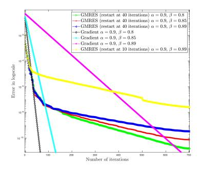
Figure 9: **Experiment 3.** Graph of convergence in  $\ell^2$ -norm : GMRES and preconditioned gradient method (Algorithm 4).
