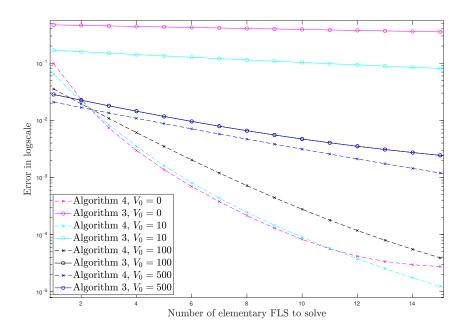
Figure 4: **Experiment 1b.**  $\ell^2$ -norm error in logscale as a function of the number of standard FLS to solve (8) with the preconditioned gradient method (Algorithm 4; with  $\rho = 0.5$  and  $\beta_{iPiano} = 0$ ) and the standard gradient method (Algorithm 3; with  $\rho = 0.5$ ).
