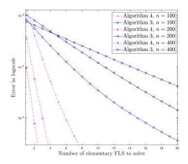
Figure 5: **Experiment 1b.**  $\ell^2$ -norm error in logscale as a function of the number of standard FLS to solve (8) with the preconditioned gradient method (Algorithm 4; with  $\rho = 0.5$  and  $\beta_{iPiano} = 0$ ) and the standard gradient method (Algorithm 3; with  $\rho = 0.5$ ) where  $\alpha = 0.75$  and  $\beta = 0.25$ , and for n = 100, 200, 400.
