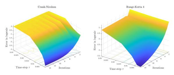
Figure 2: **Example 1a.**  $\ell^2$ -norm error in logscale as a function of the time-step  $\Delta \tau$  and iteration k of the preconditioned gradient (Algorithm 4; with  $\rho = 1$  and  $\beta_{iPiano} = 0$ ) with CN (Left) and RK4 (Right).
