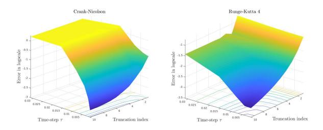
Figure 3: **Example 1a.**  $\ell^2$ -norm error in logscale as a function of the time-step  $\Delta \tau$  and truncation index M in the Taylor's series expansion with CN (Left) and RK4 (Right).
