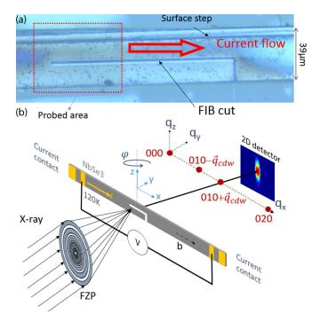
FIG. 1. (a) Optical image of the NbSe<sub>3</sub> sample showing the line cut made by the FIB, the presence of one step on the surface, and the area probed by the focused x-ray beam with 1  $\mu$ m steps. (b) Schematic drawing of the experimental setup. The sample frame is rotated with respect to the laboratory frame by an angle  $\varphi$ . The CDW is along the  $q_x$  direction, which corresponds to the  $\vec{b}$  axis of NbSe<sub>3</sub>.
