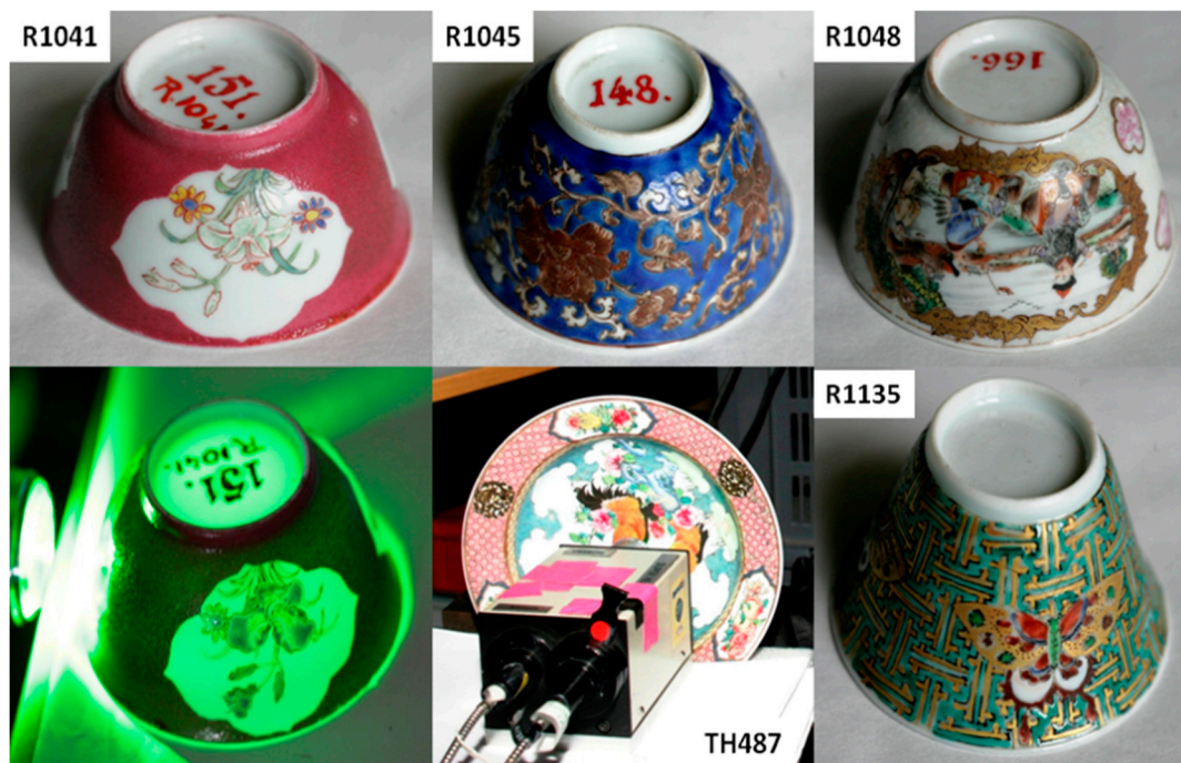
Figure 1. The cups and plate analyzed. The remote head with optic fibers connected to the laser source and the spectrometer is shown at the bottom. A laser focusing on the R1041 cup exhibits the high translucency of the porcelain (see Table 1 for details).
