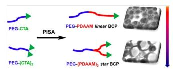
**Figure 7.** A(B)<sub>2</sub> star architecture promoting the formation of complex morphologies compared to linear diblock copolymers. Reprinted with permission from reference <sup>[234]</sup> Copyright 2017, American Chemical Society.
