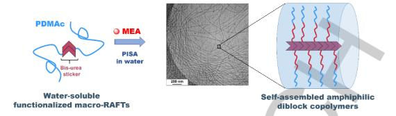
**Figure 8.** Using bis-urea functional macro-RAFT agent for "templated PISA" in water. Reprinted with permission from reference <sup>[241]</sup>. Copyright 2018, Wiley.
