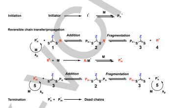
Figure 1. Reversible addition-fragmentation chain transfer (RAFT) process.
