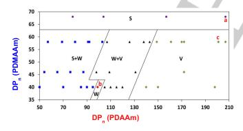
**Figure 6.** Phase diagram constructed for a series of PDMAAm-*b*-PDAAm diblock copolymer nanoobjects. S = spheres, S + W = mixed spheres and worms, W = worms, W + V = mixed worms and vesicles and V = vesicles. Reprinted with permission from reference <sup>[170]</sup> Copyright 2017, American Chemical Society.
