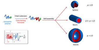
Figure 2. RAFT-mediated polymerization-induced self-assembly and illustration of the packing parameter p (by analogy to surfactants, a is the area of the hydrophilic segment and v and l are the volume and length of the hydrophobic segment) and the impact of the solvophobic block molar mass on the packing parameter/morphology.
