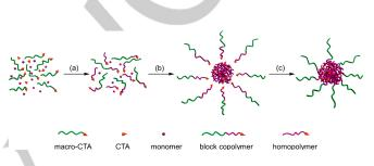
Figure 3. Polymerization-induced cooperative assembly (PICA). Reprinted with permission from reference <sup>[104]</sup> Copyright 2017, American Chemical Society.
