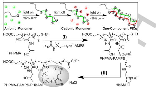
(I) [AMPS]<sub>0</sub> : [PHPMA<sub>56</sub>]<sub>0</sub> : [SPTP]<sub>0</sub> = *n* : 1 : 0.20, 25% solids, water, pH 2.5, 25°C, *hv*, 1.5 h (>99% conv) (II) add HisAM monomer to [HisAM]<sub>0</sub> : [AMPS]<sub>0</sub> = 1:1, 25% solids, water, pH 2.5, 25°C, *hv*, 3 h (>99% conv)
