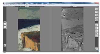
Fig. 1: Screenshot of the image database software, on the left is a photograph of a section of the painting, on the right is a 4<sup>th</sup> principal component fusion of the THz peak to peak transmission amplitude and the x-ray images.
