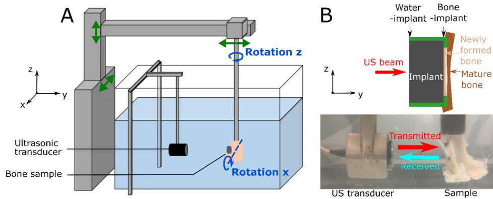
**Figure 2.** (A) Schematic representation of the quantitative ultrasonic device. The green arrows indicate the translation of each component. (B) Photo of the measurement set-up including the ultrasonic transducer acting as an emitter-receiver and the sample. The top schematic view of the implant indicates the positions of the water-implant and the bone-implant interfaces.
