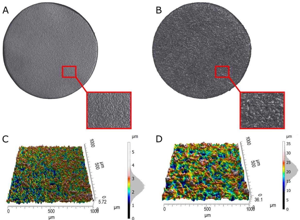
**Figure 4.** Example of implant surfaces sandblasted with (A) 25  $\mu\text{m}$  diameter particles (S series) and (B) 250  $\mu\text{m}$  diameter particles (R series). (C, D) Corresponding topographical results of  $1 \times 1 \text{ mm}^2$  maps, and distribution of the measured peaks heights (Gaussian distribution on the right-handed scale).
