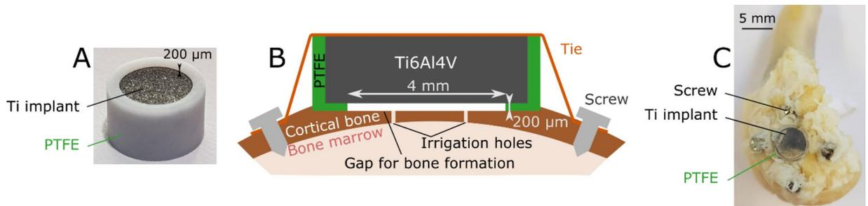
**Figure 1.** (A) Dedicated experimental model, designed as a coin-shaped implant, presented upside down—the bone chamber is visible (example of an implant from the R series). (B) Schematic cross-sectional view of the model once implanted, with the 200 µm-thick bone chamber below the implant. (C) Medial view of an implanted distal femur, after sacrifice.
