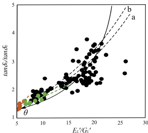
Fig. 2: A comparison of the present data with literature (Obataya et al. 2000, the figure has been revised) for the correlation of  $\tan \delta_G/\tan \delta_L$  and  $E_L'/G_L'$ . Black (literature data): the dots are the experimental values for spruce; (a) is the regression line for spruce; (b) is the regression line from 101 species;  $\theta$  is the cell wall model developed in the literature. Color (present data): the orange dots correspond to wavy maple; the green dots to spruce.
