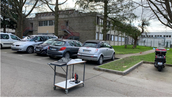
(b) A trolley shelf with the different parts of the transmission equipment at Tx location 2.
