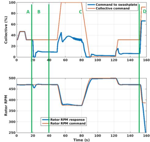
Fig. 4. Direct rotor RPM control through collective
