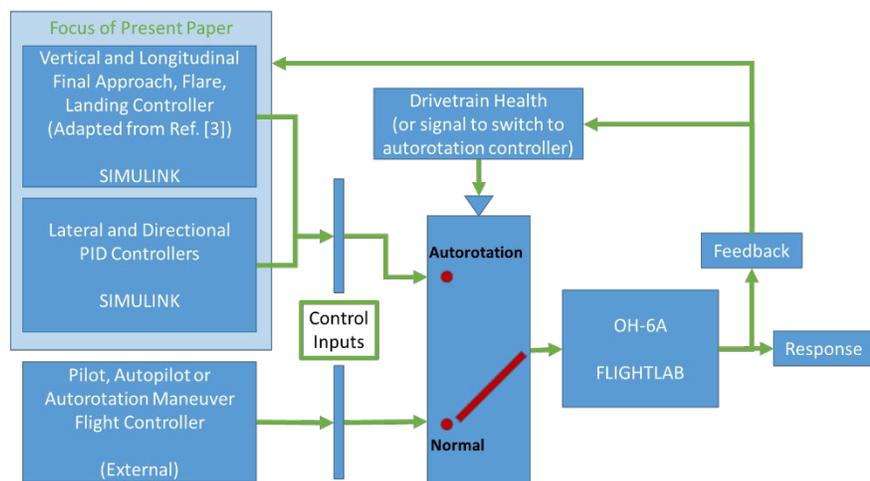
Fig. 5. Simplified block diagram of autorotation landing controller implementation
