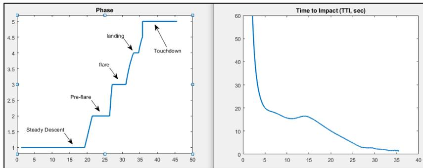
Fig. 6. Example of controller Phase and Time to Impact (TTI) parameters, baseline case
