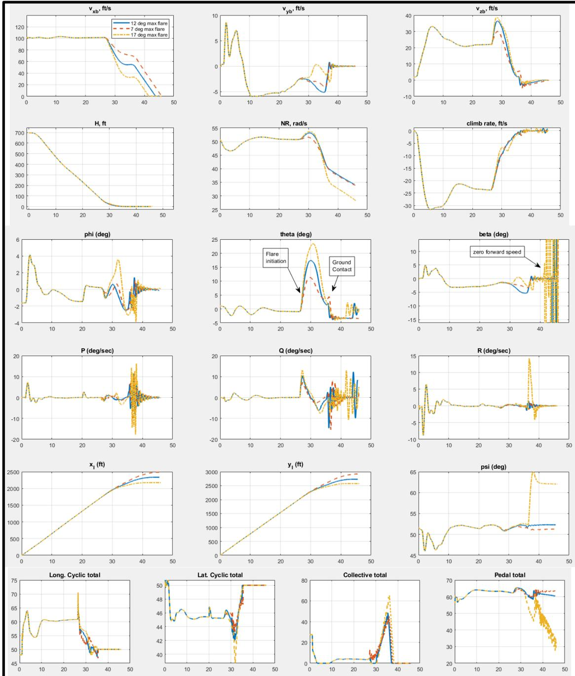
**Fig. 7** Autorotation landing controller showing the effect of varying the maximum flare pitch attitude
