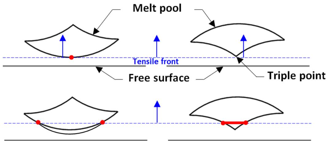
**Fig. 14.** Schematic description of the interaction between the tensile front propagating upwards from the free surface (blue dotted line) and the melt pool boundaries, after shock loading along  $-Z$  (left) or  $+Z$  (right), at two successive instants (top then bottom).
