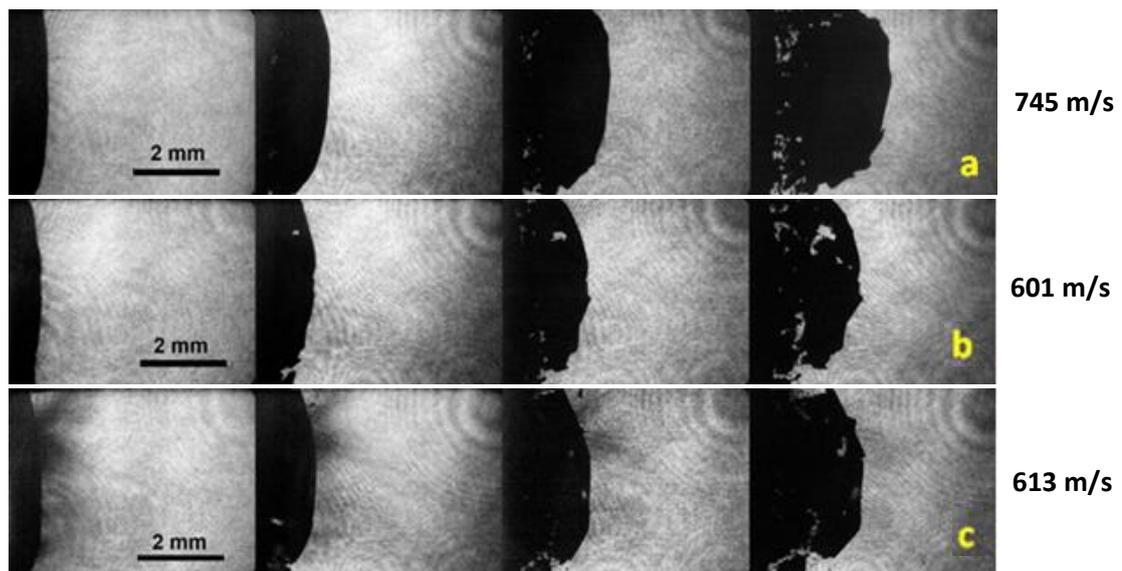
**Fig. 8.** Transverse shadowgraphs recorded at  $1\mu\text{s}$ ,  $2\mu\text{s}$ ,  $3\mu\text{s}$  and  $4\mu\text{s}$  from left to right, in (a) P1-Z, (b) P2-Z and (c) P2-XY samples with the mean velocity of the main spalled layer.
