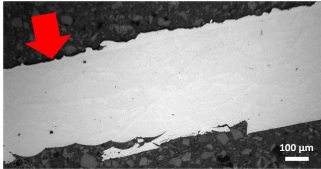
**Fig. 13.** Optical micrograph of a cross section in sample P1-Z-500-1 shocked along the  $-Z$  axis (same as Fig. 9) at the edge of the loaded zone, where two distinct spalled layers have separated from the bulk. Shock loading has been applied from top to bottom (red arrow).
