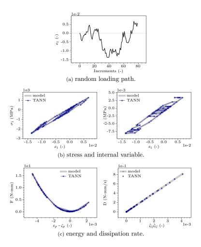
Figure 9: Predictions of TANN for a uni-axial random loading path, compared with the target constitutive model, case H-1, perfect plasticity: (a) loading path; (b) principal stress,  $\sigma_1$ , and internal variable,  $\zeta_1$ , predictions; (c) energy and dissipation rate predictions.
