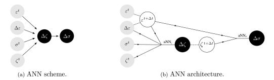
Figure 10: Schematic (a) and full architecture (b) of the network, not based on thermodynamics, standard ANNs. Inputs are highlighted in gray  $(\bullet)$ , outputs in black  $(\bullet)$ .
