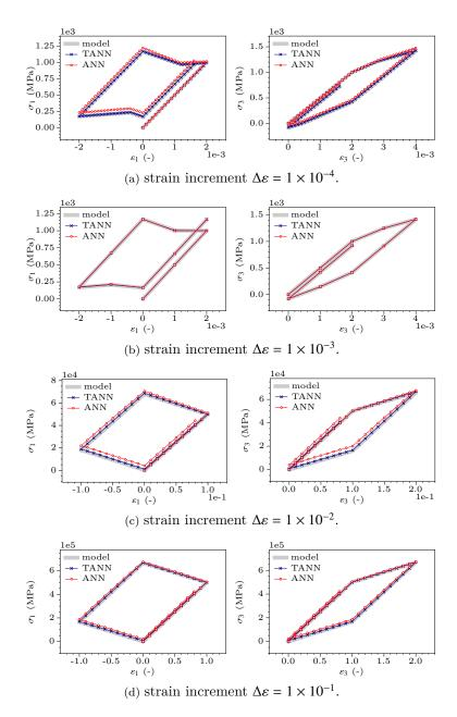
Figure 13: Comparison of the stress predictions of TANNs and standard ANNs with respect to the target values, for the tri-axial cyclic loading path, Eq. (27), for material case H-1 (perfect plasticity). Each row represents the prediction at different  $\Delta \varepsilon$  increments.
