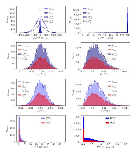
Figure 7: Sampling for material case H-1 (cf. Table 1). From top to bottom: mean and deviatoric stress (p and q); mean and deviatoric total deformation ( $\varepsilon_p$  and e); mean and deviatoric plastic deformation ( $\zeta_p$  and z); energy (F) and dissipation rate (D). Training and validation data-sets are also distinguished.
