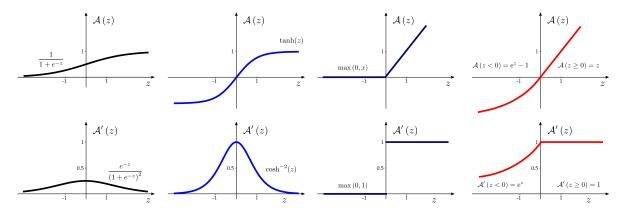
Figure 4: Some of the most common activation functions and their first-order gradient. From left to right: the logistic (sigmoid) function, the hyperbolic tangent, the Rectified Linear Unit (ReLU), and the Exponential Linear Unit (ELU).
