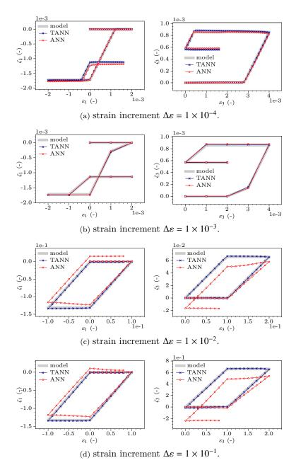
Figure 14: Comparison of the internal variable predictions of TANNs and standard ANNs with respect to the target values, for the tri-axial cyclic loading path, Eq. (27), for material case H-1 (perfect plasticity). Each row represents the prediction at different  $\Delta \varepsilon$  increments.
