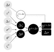
Figure 2: Schematic architecture of TANN. Inputs are highlighted in gray  $(\bullet)$ ; outputs in black,  $(\bullet)$  and  $(\blacksquare)$ ; and intermediate quantities in white  $(\bigcirc)$ . Dashed lines represent definitions, while arrows are used to denote neural network links.
