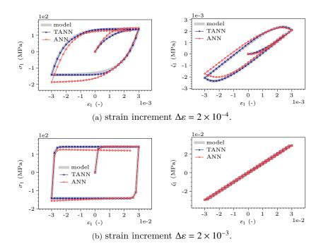
Figure 16: Comparison of the stress and internal variable predictions of TANNs and standard ANNs with respect to the target values, for a bi-axial cyclic loading path,  $\Delta \varepsilon_2 = -\Delta \varepsilon_1$ , with  $\Delta \varepsilon_1$  as in Eq. (5.2.1), for a perfect hypo-plastic material. Each row represents the predictions at different  $\Delta \varepsilon$  increments.
