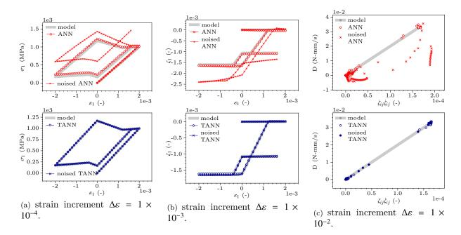
Figure 19: Influence of noise in the stress,  $\sigma_i$ , for the predictions of the stress, internal variable, and dissipation rate of TANNs and of standard ANNs with respect to the target values, for the tri-axial cyclic loading path for material case H-1 (perfect plasticity). Noise strongly affect the predictions of standard ANNs, see Fig.s 13-15.
