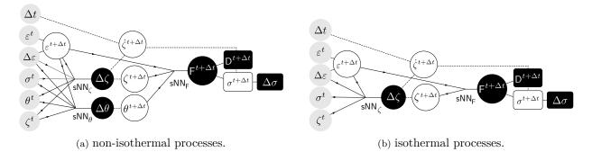
Figure 6: Architecture of TANNs: general case (a) and for isothermal processes (b). Inputs are highlighted in gray ( $\bullet$ ); outputs in black, ( $\bullet$ ) for direct ANN predictions and ( $\blacksquare$ ) for derived outputs; and intermediate quantities (definitions) are in white ( $\bigcirc$ ) and ( $\Box$ ). Relationships obtained from definitions are represented with dashed lines, while arrows denote ANNs.
