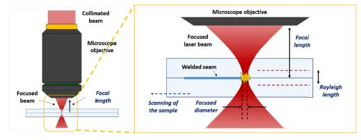
Fig. 2. Schematic view of the common glass welding process by femtosecond laser pulses using microscope objective.
