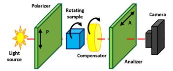
Fig. 5. Experimental setup for stress observation using photoelasticimetry.
