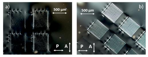
Fig. 8. Observation by photoelasticimetry of welding seams: determination of the residual stress orientation by the rotation of the sample. (500 kHz, 100 mm/s,  $3-6 \mu J$ )
