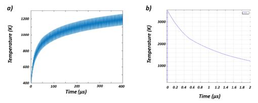
Fig. 7. Temporal temperature evolution for 3  $\mu$ J, 300 fs, 500 kHz pulses, showing: a) the slow thermal accumulation effect inside the material in the configuration with the 5 theta lens, focal length f=100 mm (Heat source:  $Z_s = 200 \ \mu m$ ,  $r_s = 4 \ \mu m$ ,), b) the fast temperature increases with a microscope objective, focal length f=10 mm (Heat source:  $Z_s = 50 \ \mu m$ ,  $r_s = 2 \ \mu m$ ).
