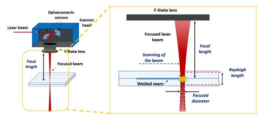
Fig. 3. Schematic view of glass welding by ultra-short laser pulses using a galvanometric head.
