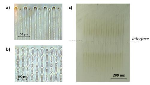
Fig. 9. Top and side views of welding seams: a) top view of homogeneous welding seams (500 kHz, 100 mm/s, 5 μJ), b) top view of inhomogeneous welding seams (2 MHz, 100 mm/s, 2.8 μJ), c) side view of homogeneous welding seams (500 kHz, 50 mm/s, 4.8 μJ).
