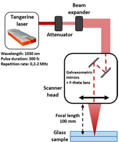
Fig. 4. Experimental setup for femtosecond laser glass welding with a long focal length focusing lens, as used in this paper.
