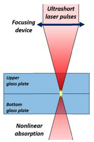
Fig. 1. Schematic view of our glass welding setup by femtosecond laser pulses.
