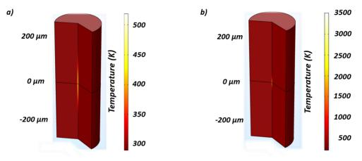
Fig. 6. Temperature distribution inside glass induced by the absorption of the first laser pulse, before thermal diffusion (1030 nm, 3  $\mu$ J, 300 fs), a) Heat source:  $Z_s = 200 \,\mu m$ ,  $r_s = 4 \,\mu m$ , generated by a scanner head, focal length f = 100 mm and b) Heat source:  $Z_s = 50 \,\mu m$ ,  $r_s = 2 \,\mu m$ , generated by an optical microscope, focal length f = 10 mm.
