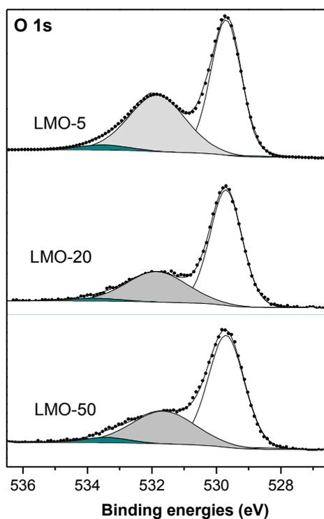
**Figure 7.** O 1s core peaks for the three  $\text{Li}_2\text{MnO}_3$  samples with 5%, 20% and 50% of stacking faults after adsorption. The white, grey and green components correspond to the structural oxygen atoms, the surface oxygen atoms and the oxygen atoms of adsorbed species, respectively.
