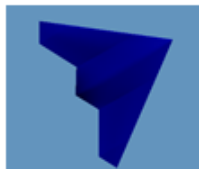
group 2 : Lower part of the Wings and fuselage T_{avg,2} = 282 \text{ K} \epsilon_2 = 0,6 Directional, Niratam
