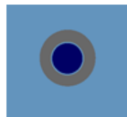
group 6 : Disc exhaust entry T_{avg,6} = 627 \text{ K} \epsilon_6 = 0,99 Lambertian
