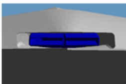
group 5 : Inner part of exhaust duct T_{avg,5} = 350 \text{ K} \epsilon_5 = 0,95 Lambertian
