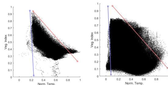
**Fig. 2.** 2D scatterplots of the Vegetation Index (OSAVI) vs. the normalized brightness temperature as obtained from the manned aircraft (left) and from the UAV (right). The wet edge is in blue and the dry edge is in red.
