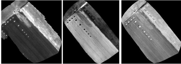
Fig. 4. Results obtained with UAV at 16h. OSAVI (left) Temperature (middle), inferred Water index (right).
