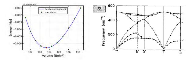
**Fig. 1:** (Left) Energy versus unit-cell volume for silver. DFT energy data points are fitted by some clever functional form (Birch-Murnagham fit). The energy minimum gives the equilibrium volume and related lattice parameter as well as interatomic distances that can be compared to experiment (courtesy http://exciting-code.org/beryllium-volume-optimization-for-cubic-systems). (Right) Calculated LDA versus experimental phonon dispersion for silicon (from Ref. [13]).
