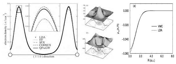
**Fig. 2:** (Left) Charge density for solid argon along an interatomic bond comparing LDA with the so-called quasiparticle self-consistent QPscGW approximation (from Ref. [14]). (Center and Right) LDA versus variational Monte Carlo (VMC) one-body density matrix and spherically averaged XC hole  $\rho_{XC}(\mathbf{r}; R)$  for Silicon (from Ref. [15]).
