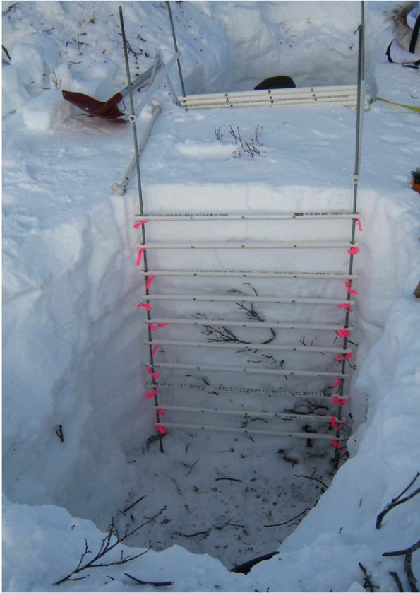
FIG. 2. Photograph taken during shrub sampling in January 2016. Snow had to be carefully removed to cut branches within each of the 10-cm strata, which are marked by the horizontal plastic bars in the photograph.
