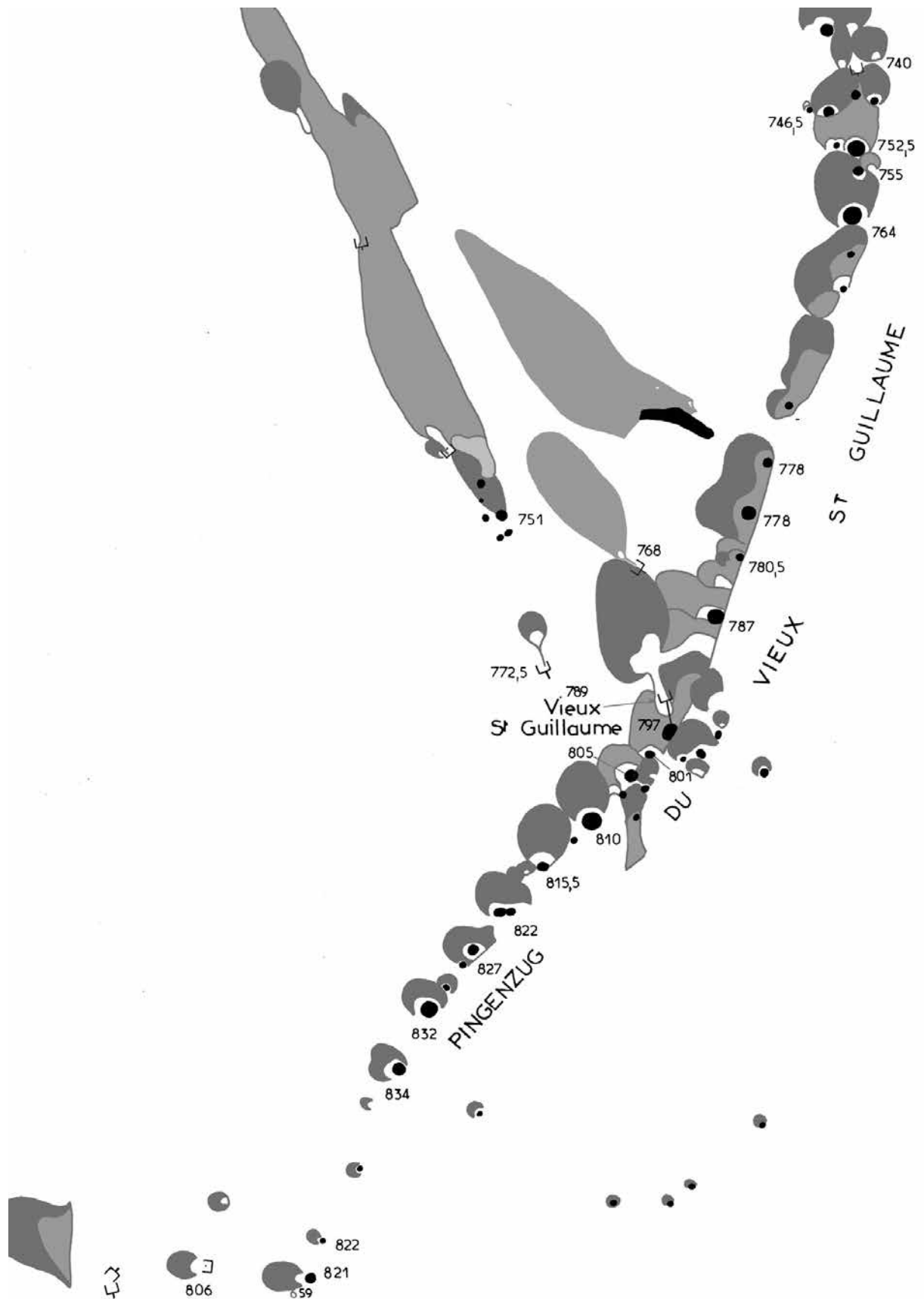
Fig. 5: Map of the upper part of the Altenberg area, showing the open shafts ( Pingen ) and their tailings, and the location of Vieux-Saint-Guillaume and Vieux-Rimpy mines (below on the left, two galleries).
