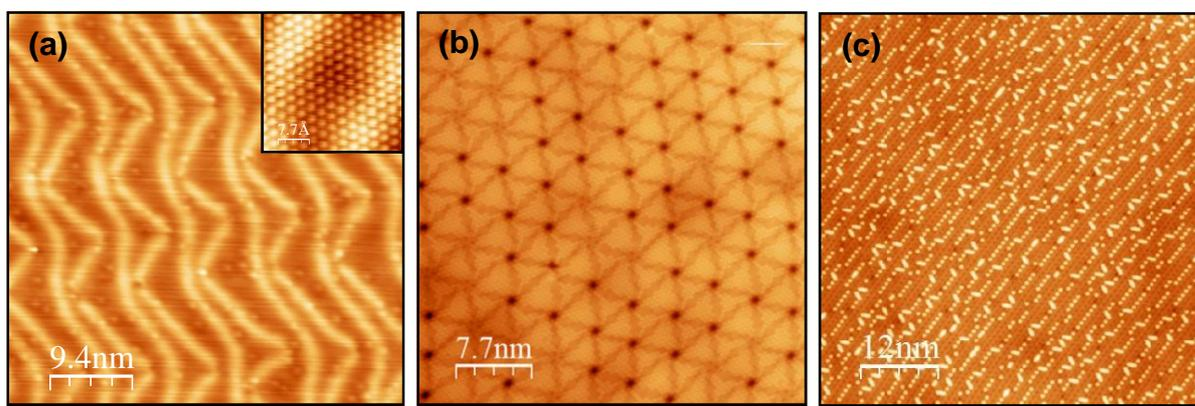
**Fig.1:** (a) Large-scale STM image of clean Au(111) surface, showing the herringbone reconstruction ( $U=-0.7V$ ,  $I=1.0nA$ ) and insert displays the associated image with atomic resolution. (b,c) Large-scale images measured on Au(111) covered by 0.33 ML and 0.5 ML of Te, respectively.
