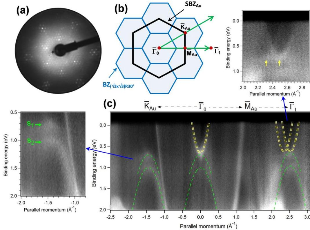
**Fig.7:** (a) LEED pattern and (b) the corresponding schematic of the SBZs of the  $(\sqrt{3}\times\sqrt{3})R30^\circ$  reconstruction obtained after deposition of 0.33ML of Te on  $\text{Au}(111)$  surface. (c) ARPES mapping of band structure along  $K$ - $\Gamma$ - $M$ - $\Gamma$  directions measured also on  $\text{Au}(111)$  covered by 0.33 ML of Te. The ARPES data have been recorded at  $T=100\text{K}$  with a photon energy of 60eV and the LEED pattern measured at energy of 80 eV.
