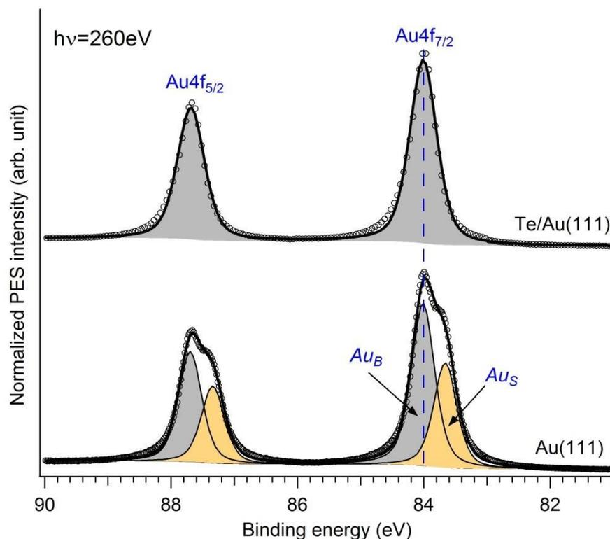
**Fig.4:** Core level  $Au4f$  XPS spectra recorded at normal emission before and after deposition of 0.5ML of Te on  $Au(111)$ . As shown, the deconvolution of these spectra yields to two contributions for the clean substrate,  $Au_B$  stands the bulk and  $Au_S$  the surface, while only the  $Au_B$  one is present after growing Te on the surface.
