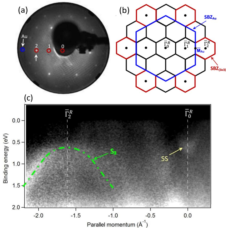
**Fig.8:** (a) LEED pattern obtained on Au(111) surface covered by 0.5ML of Te, showing (3x3) reconstruction and (b) the corresponding surface Brillouin zone. (c) ARPES results obtained on the same surface along the  $\Gamma M$  directions of the Au(111) SBZ.
