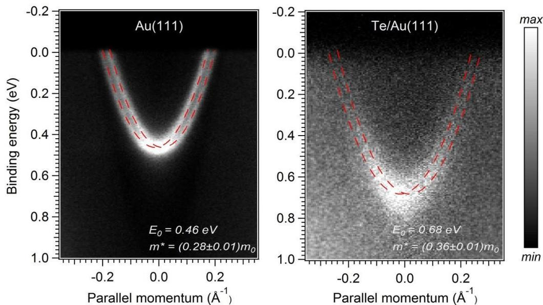
**Fig.6:** Shockley state bands measured by ARPES on pristine Au(111) (left panel) and on Au(111) covered by 0.33 ML of Te (right panel). The ARPES data have been recorded at normal emission along  $\Gamma$ -M direction and at  $T=100K$  with a photon energy of 60eV.
