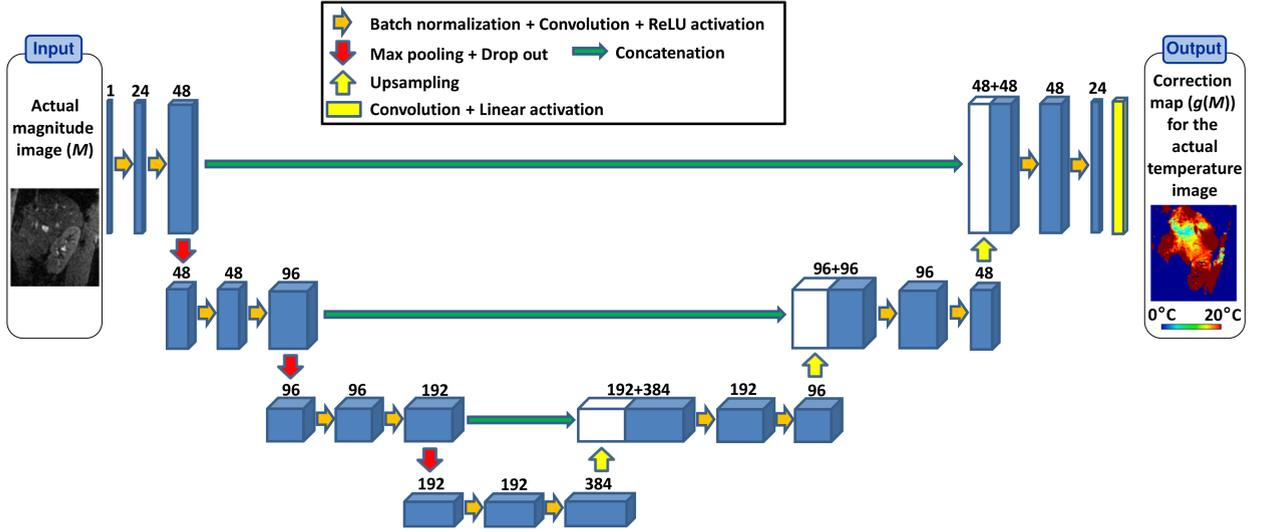
**Figure 3:** Architecture of the deep neural network proposed for learning motion-related errors in MR-thermometry before heating (red block in figure 2). The most recent magnitude image (*i.e.*,  $M$ ) is used as a single input channel. The CNN-model constructs a correction map (noted  $g(M)$ ) for the current temperature map. Each block of the CNN is composed of batch normalization, convolution and ReLU activation. The number of  $3 \times 3$  filters is indicated on the top of each block.
