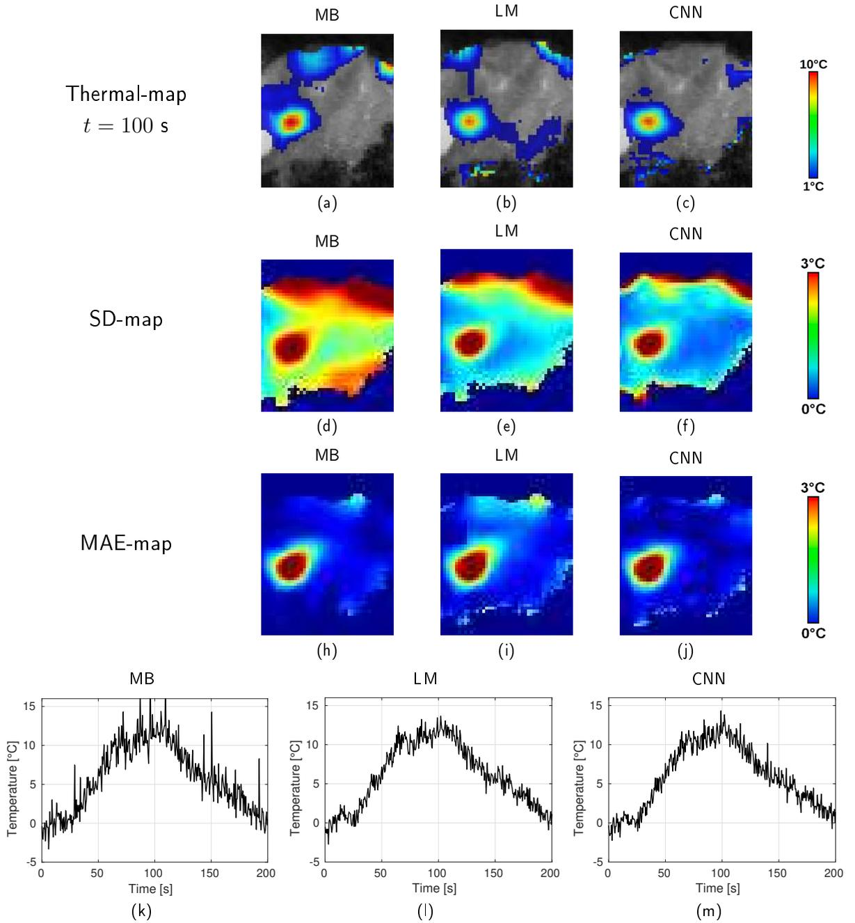
**Figure 8:** MR thermometry results obtained in a porcine liver during HIFU heating: (first row) Temperature maps obtained after 80 s of heating ( $t = 100s$ ) overlaid on the anatomic image, (second row) temporal standard deviation map, (third row) mean absolute error map, and (bottom row) temporal evolution of the temperature in a single voxel located at the focal point position. Results are reported using LUT (left), LM (middle) and CNN (right).
