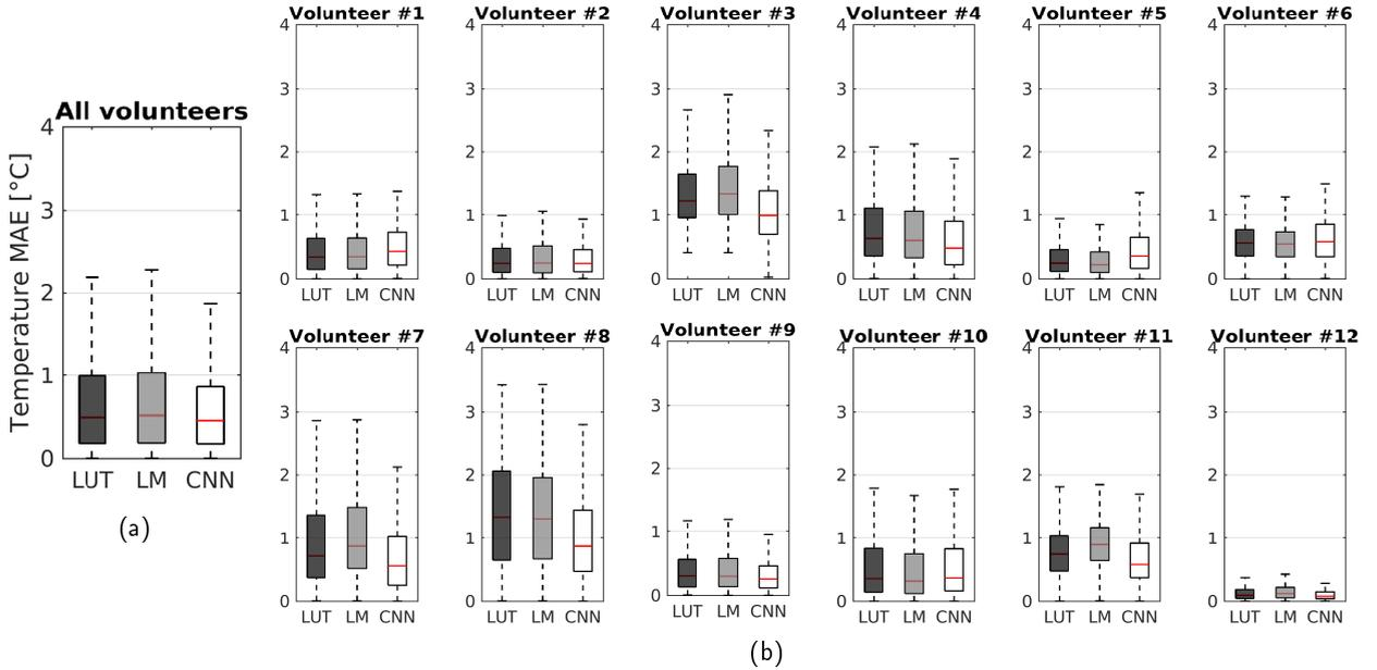
**Figure 6:** Comparison of temperature accuracy obtained using LUT, LM and CNN in the liver of free-breathing healthy volunteers during 4 minutes and 40 seconds of MR-thermometry. Similar to figures 4 and 6,  $N = 200$  images were used for training. Box-and-whisker plots of the temporal temperature mean absolute error are shown using LUT (dark gray box), LM (light gray box) and CNN (white box): (a) group analysis over the 12 volunteers, (b) volunteer-wise analysis.
