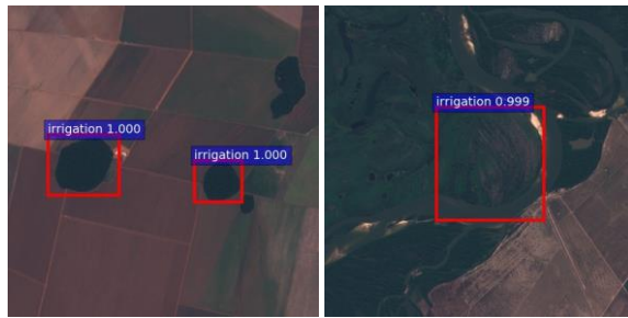
Figure 8. Examples of false detections by PVANET
