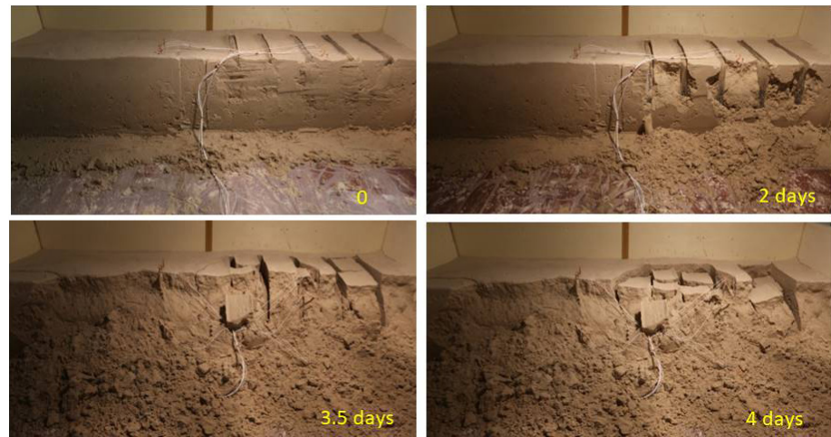
Figure 2. RTS experiment no. 1 (with ice wedges) of 2.5 m × 2.5 wide and 0.5 m height showing on the left side a homogeneous frozen soil and on the right side the same frozen soil (saturated fine sand) with additional artificial ice wedges. The thick vertical brown line on the top of each photo separates left from right part. Active erosion due to the presence of ice wedges is observed on the right side of the experiment. White cables correspond to temperature sensors.
