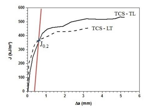
Fig. 2: *J*-d*a* curves of two TCS compact tension (CT) specimens;
