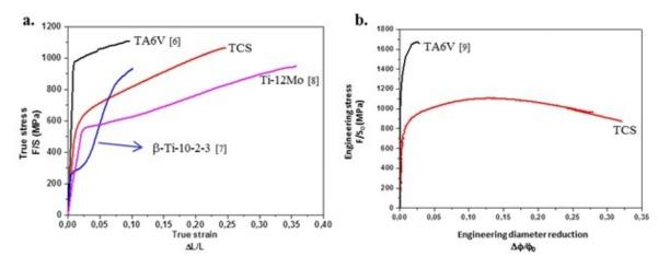
Fig. 1: a. Uniaxial true stress-true strain tensile curves of four Ti alloys [6][7][8];
