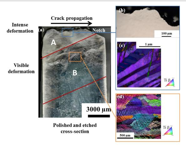
Fig. 3: Optical microscopy image of a. the etched mid-thickness cross-section of a Charpy specimen, b. the top of the cross section to evidence no damage; c. PACOM-TEM orientation imaging micrograph of a thin foil taken across the fracture surface the same Charpy specimen; d. EBSD orientation imaging micrograph below the fracture surface; inverse pole figure maps (tensile direction) are superimposed with Image Quality (IQ)
