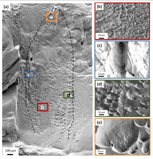
Fig. 4: a-e. SEM images under secondary electron mode of a. macro-cavity (delimited by black dashed line) composed of b. two-sized dimples, c. d. vein-like areas composed of aligned, incompletely closed dimples; e. plasticity ridges inside a dimple
