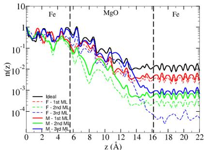
FIG. 9. Spin up  $\Delta_1$  scattering state distribution along the transport direction  $z$  for various vacancy configurations of Fe/F-MgO(5ML)/Fe and Fe/M-MgO(5ML)/Fe in the MTJ's P magnetic state. All the data are normalized and the same logarithmic scale is used.
