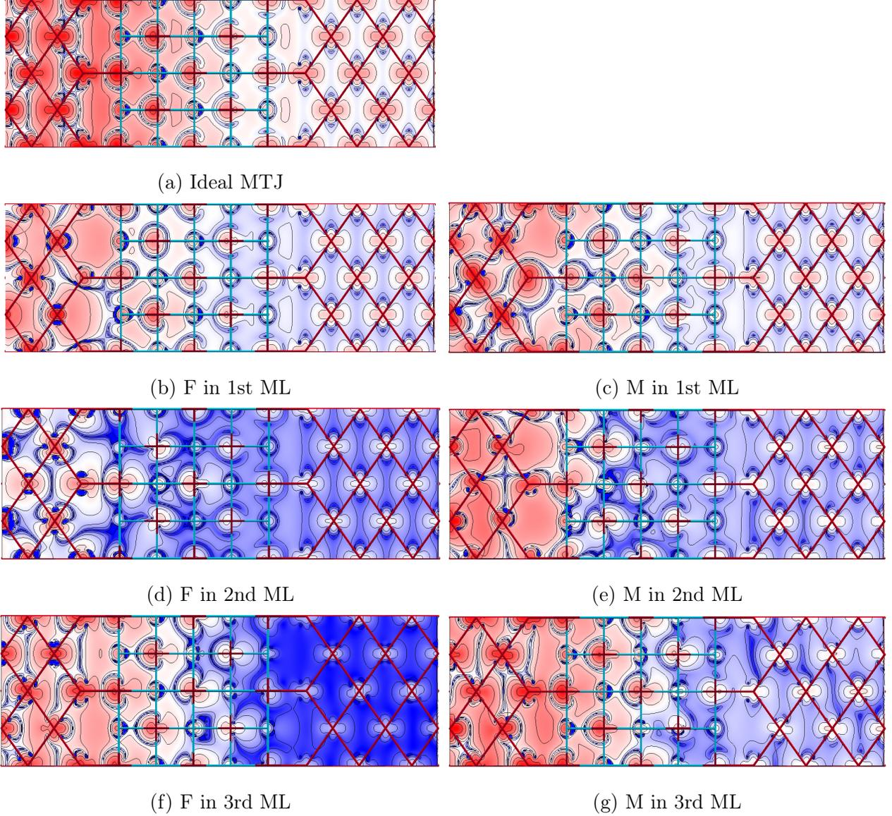
FIG. 10. 2D representation of the spin up  $\Delta_1$  scattering states in the  $x, z$  plane for various vacancy configurations of . All the data are normalized and the same logarithmic scale is used (see Fig. 9.
