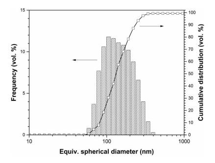
Figure 4: Granulometric distributions of the ZrO<sub>2</sub> powders synthesized by means of a zirconium-doped ammonium nitrate-based explosive emulsion detonation.
