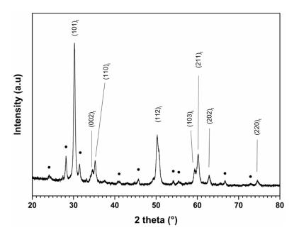
Figure 1: XRD pattern of the zirconium (IV) oxide sample  $(ZrO_2)$  synthesized by means of a zirconiumdoped ammonium nitrate-based explosive emulsion detonation. The symbols t and  $\bullet$  are attributed to the tetragonal and monoclinic structures, respectively.
