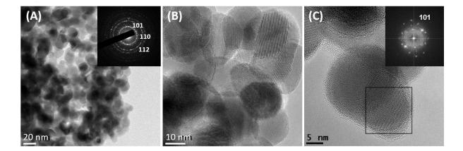
Figure 2: TEM images of the ZrO<sub>2</sub> powder synthesized by means of a zirconium-doped ammonium nitrate-based explosive emulsion detonation. a) Bright field TEM image combined with the SAED pattern using a aperture of 150 nm b) and c) HRTEM images showing the high cristallinity of the nanograins specially on c) with the FFT of the HRTEM image corresponding to the (101) planes of ZrO<sub>2</sub> tetragonal.
