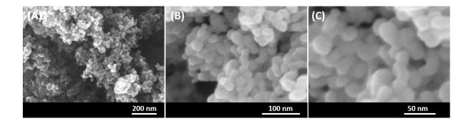
Figure 3: SEM images in secondary electron mode of the ZrO<sub>2</sub> powder synthesized by means of a zirconium-doped ammonium nitrate-based explosive emulsion detonation a) global view b) and c) same view with higher magnification.
