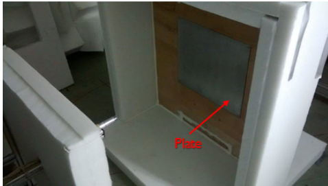
Figure 5. Baffled simply supported panel
