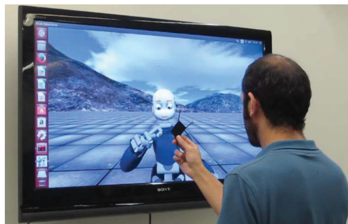
Fig 4. The experimental setup. The avatar is displayed on a big screen (46 inches). The avatar led the mirror game and the participant followed the avatar's hand motions. The participant held a marker for motion tracking purposes.
