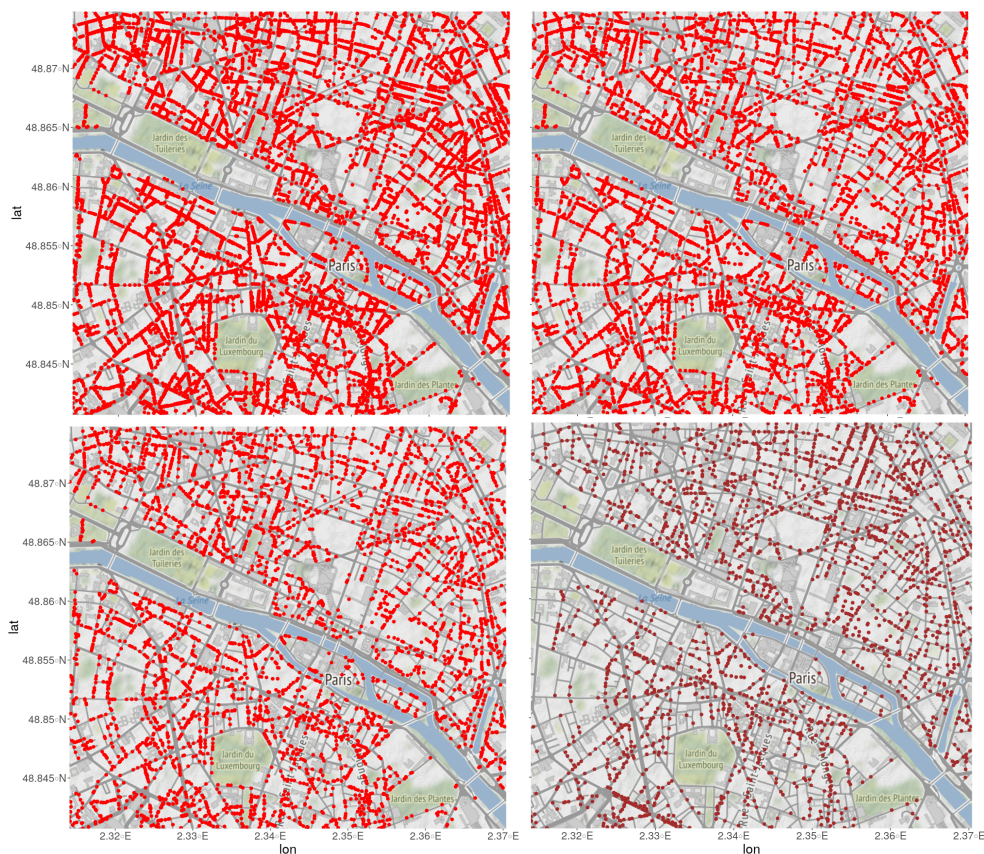
Fig. 5: Optimal parking cover solution for the weighted hypergraph given R = 10 (upper-left), R = 50 (upper-right) and R = 100 meters (lower-left), in addition to the FLZ parking spots implemented by local authorities (lower-left).
