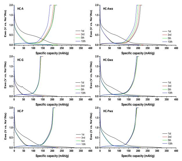
**Figure 9.** GCPL profiles of 1<sup>st</sup>, 3<sup>rd</sup>, 5<sup>th</sup> and 10<sup>th</sup> cycles. Comparison between pristine (left) and washed (right) HCs cycled at C/10 rate.
