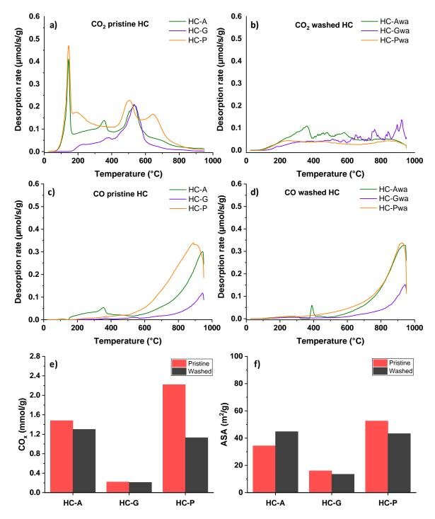
**Figure 6.**  $CO_2$  and CO TPD-MS desorption profiles for pristine (a, c) and washed (b, d) hard carbons e) Desorbed quantities of oxygen-based functional groups,  $CO_x$  (CO + CO<sub>2</sub>) and f) Active Surface Area of pristine and washed hard carbon materials after the TT.
