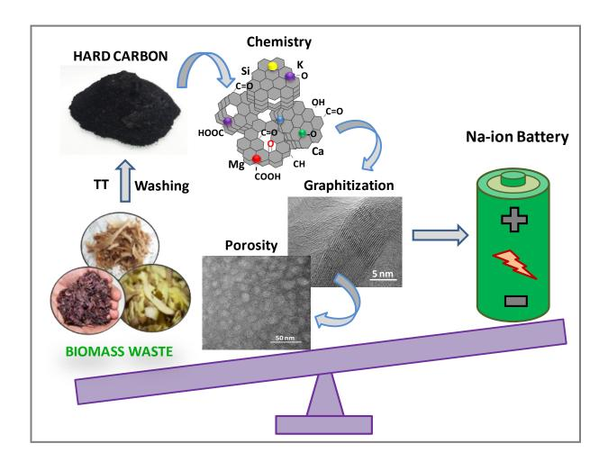
Biomass waste inorganic impurities impact the structure, the porosity and the surface chemistry of hard carbon and their performance as anode in Na-ion batteries.
