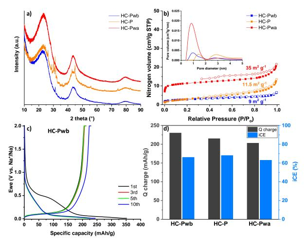
**Figure 11.** a) XRD data and b) N<sub>2</sub> adsorption-desorption isotherms and pore size distribution (inset) of HC-Pwb, HC-P and HC-Pwa potato peel derived hard carbons. c) GCPL profiles for HC-Pwb and d) Reversible capacity and iCE of HC-Pwb, HC-P and HC-Pwa materials.
