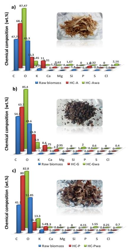
**Figure 2.** Chemical composition determined by EDX for biomass precursors, hard carbons and washed hard carbons after pyrolysis: a) asparagus, b) grape and c) potato. *In-set*: images of raw biomass precursors.
