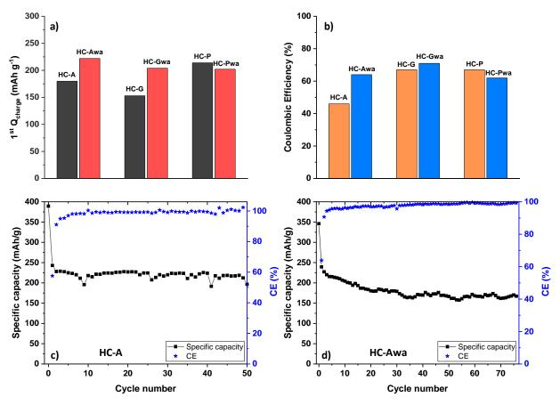
**Figure 10.** a) First cycle charge capacity and b) initial Coulombic efficiency of the hard carbon materials. Long term cycling along with CE of asparagus derived HC: c) pristine and d) washed.
