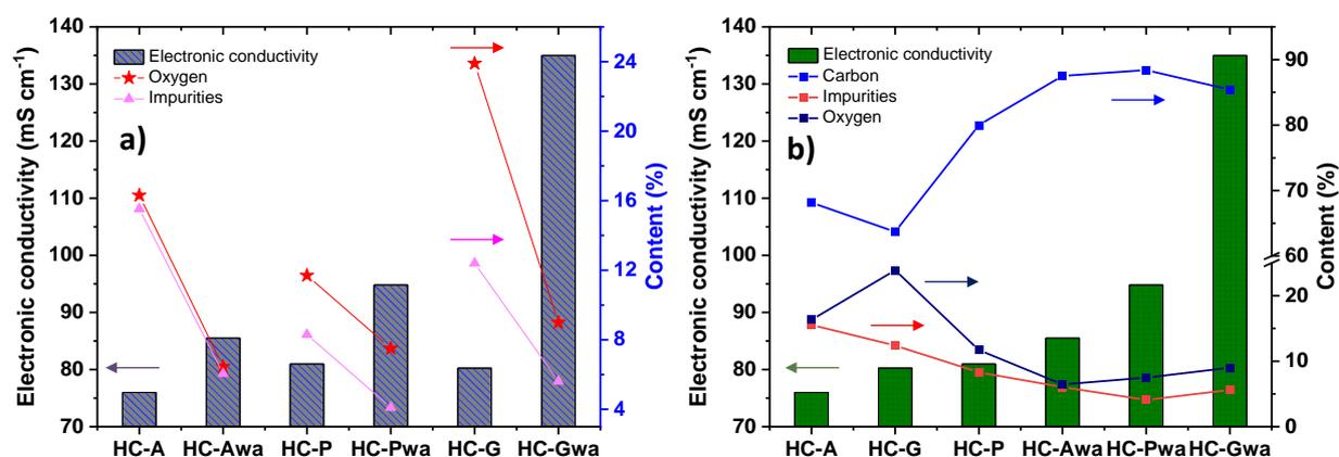
Figure 7. a) Electronic conductivity of the pristine and washed hard carbon materials versus oxygen and impurities content. b) Ascending evolution of the electronic conductivity and the correlations with the carbon, oxygen and impurities contents.
