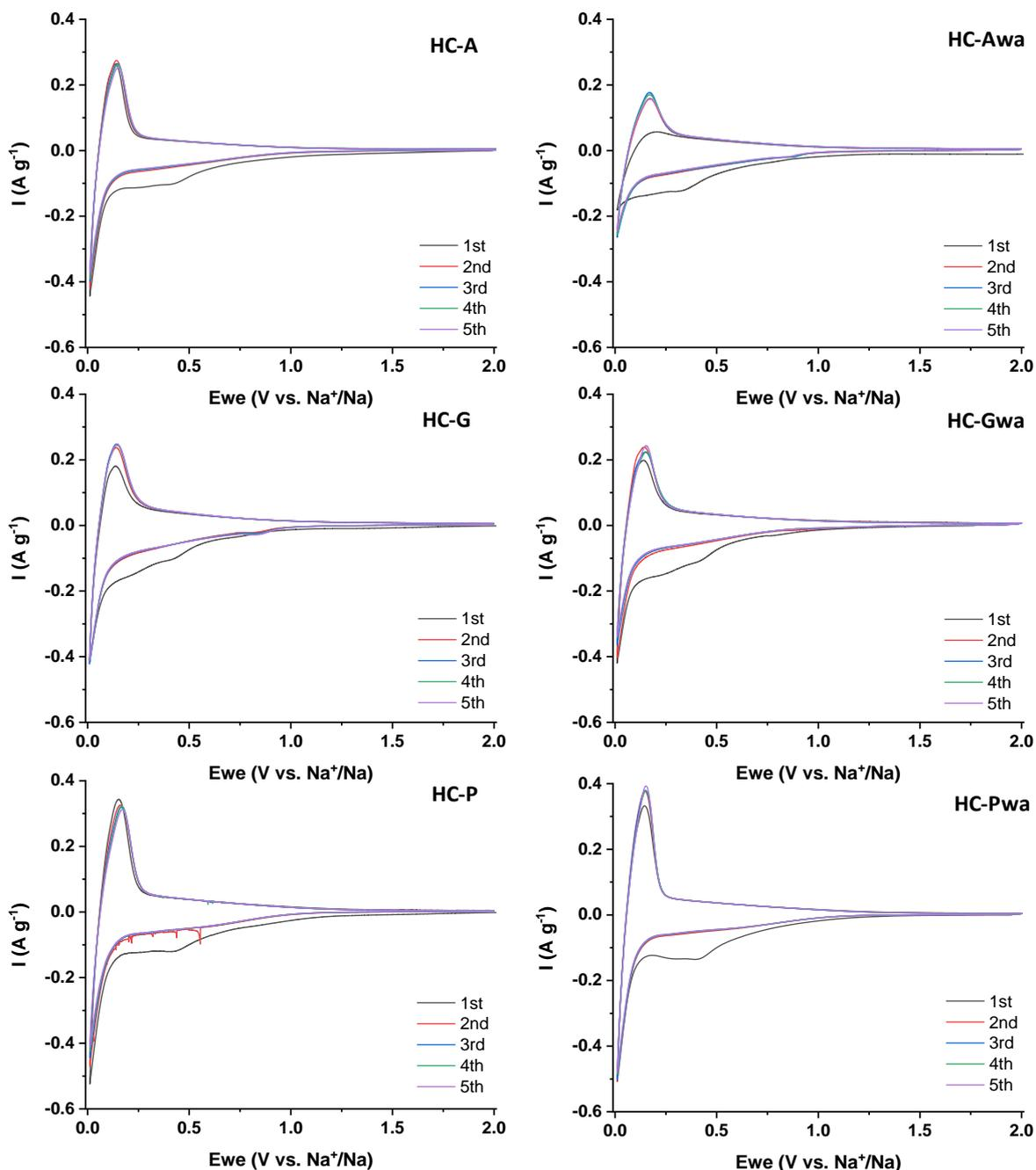
**Figure 8.** Cyclic voltammograms of pristine (left) and washed biowaste (right) derived HCs from 2-electrodes tests.
