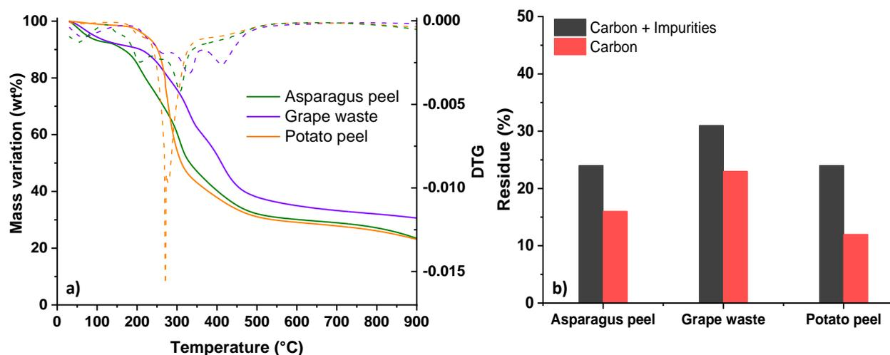
**Figure 1.** a) TGA/DTG curves under nitrogen of the different biomasses; b) Residue yield obtained from the raw biomass conversion into carbon at 900°C and the carbon yield obtained by subtracting the amount of impurities obtained following materials oxidation under air by TGA.
