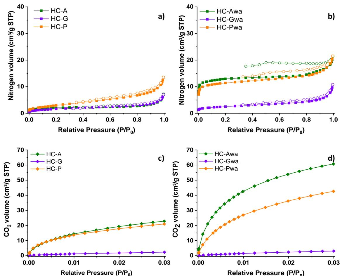
**Figure 5.** N<sub>2</sub> adsorption-desorption isotherms (a, b) and CO<sub>2</sub> adsorption isotherms (c, d) of pristine (left) and washed (right) HCs
