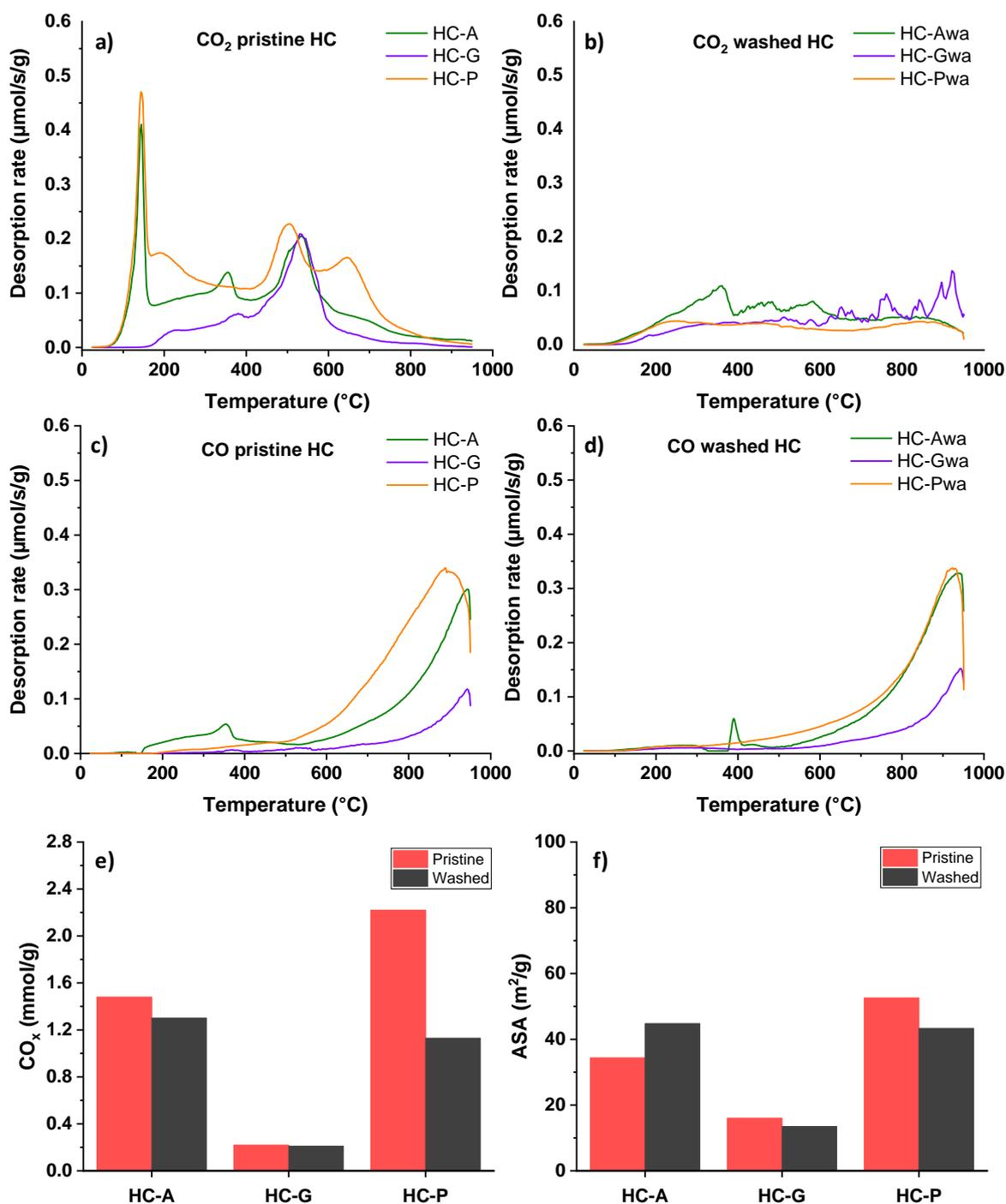
**Figure 6.** CO<sub>2</sub> and CO TPD-MS desorption profiles for pristine (a, c) and washed (b, d) hard carbons e) Desorbed quantities of oxygen-based functional groups, CO<sub>x</sub> (CO + CO<sub>2</sub>) and f) Active Surface Area of pristine and washed hard carbon materials after the TT.
