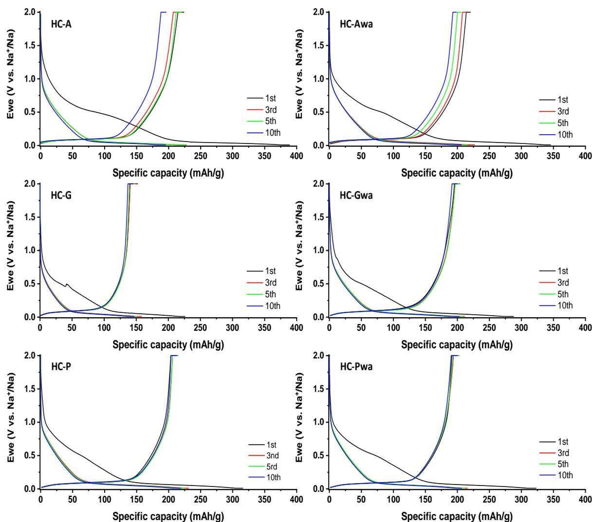
**Figure 9.** GCPL profiles of 1<sup>st</sup>, 3<sup>rd</sup>, 5<sup>th</sup> and 10<sup>th</sup> cycles. Comparison between pristine (left) and washed (right) HCs cycled at C/10 rate.
