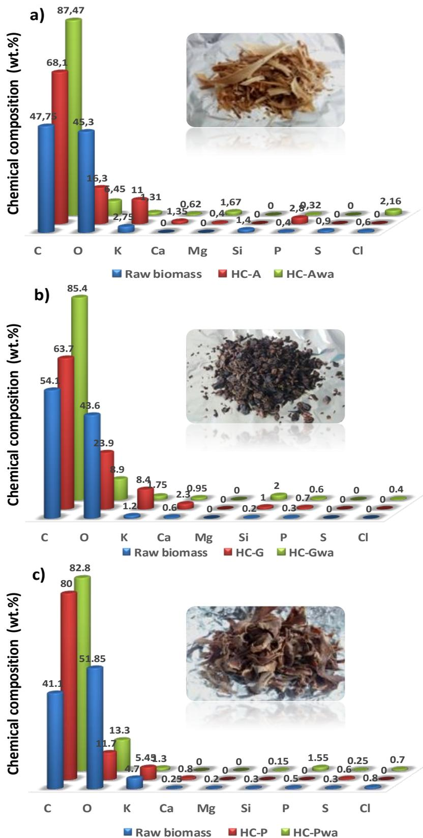
**Figure 2.** Chemical composition determined by EDX for biomass precursors, hard carbons and washed hard carbons after pyrolysis: a) asparagus, b) grape and c) potato. *In-set*: images of raw biomass precursors.
