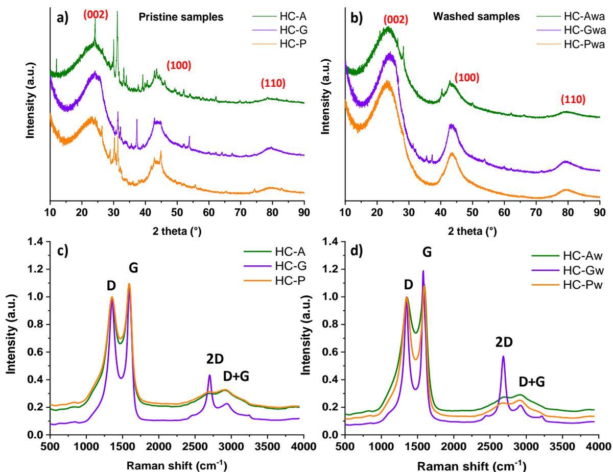
**Figure 3.** XRD diffractogram of (a) HC materials heat-treated at 1300°C along with b) washed after TT hard carbon materials. Raman spectra normalized to D band intensity of pristine (c) and washed (d) biomass derived hard carbons.
