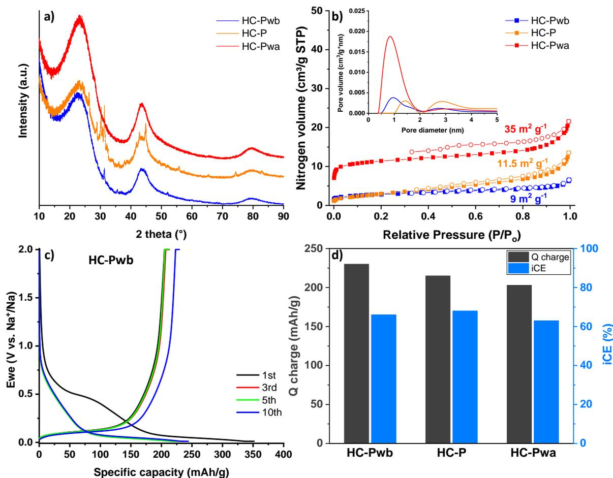
**Figure 11.** a) XRD data and b)  $N_2$  adsorption-desorption isotherms and pore size distribution (inset) of HC-Pwb, HC-P and HC-Pwa potato peel derived hard carbons. c) GCPL profiles for HC-Pwb and d) Reversible capacity and iCE of HC-Pwb, HC-P and HC-Pwa materials.
