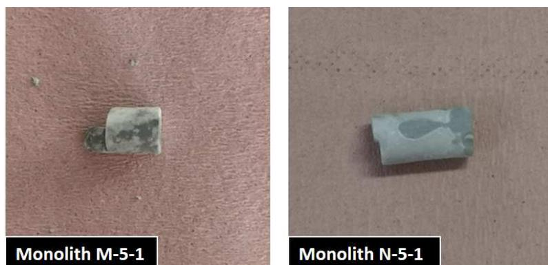
**Figure 13.** Photographs of the synthesized monoliths M-5-1 and N-5-1 after mercury intrusion-extrusion experiments
