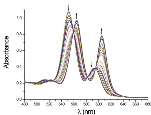
**Figure 2.** UV-Vis spectroscopic titration of dimer **2** with DABCO in CH<sub>2</sub>Cl<sub>2</sub> at rt. Spectral changes of **2** on addition of DABCO at rt: **2**] =  $3.10^{-5}$  M, concentration ratio [DABCO] / **2**] = 0 to 100.
