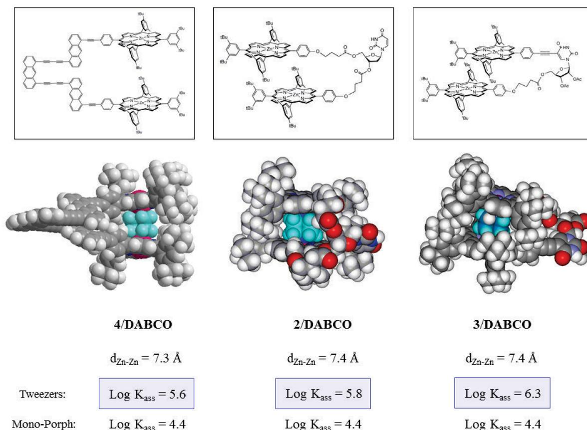
**Figure 4.** Molecular modeling of dimers **4**, **2** and **3** and their 1/1 complexes: **4/DABCO**, **2/DABCO**, **3/DABCO**. The center to center distance between the two porphyrins is ~ 7.4 Å in all dimers. Geometry optimizations have been done by molecular mechanics with the ESFF force field using the computer program Spartan.
