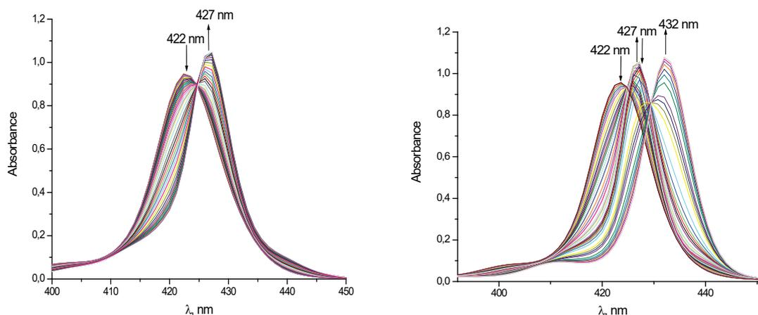
**Figure 6.** UV-visible titration of bis-porphyrinic tweezer **5** with DABCO in  $\text{CH}_2\text{Cl}_2$  at rt. On the left hand side first part of the titration and on the right the complete titration.
