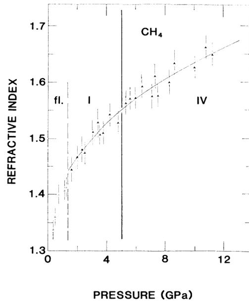
FIG. 5. Refractive index as a function of pressure at  $\lambda = 514.5$  nm and room temperature. The open triangles are in the fluid and the solid ones are in the solid. The continuous line is the result of the fit using Eq. (2).
