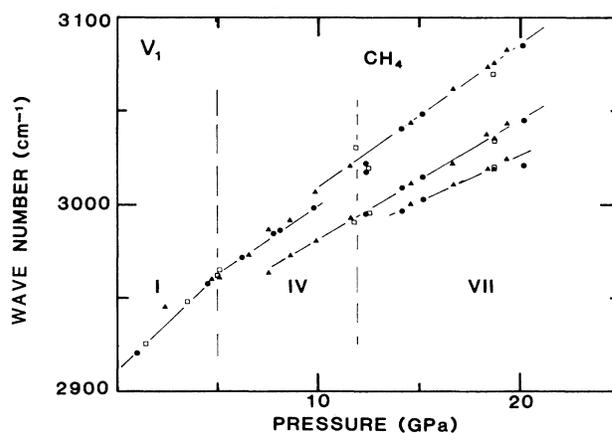
FIG. 2. Summary of the evolution of the  $\nu_1$  mode with pressure. The points are obtained at increasing pressure, and the triangles by decreasing it. The open squares are from Ref. 5. The continuous lines are used to calculate the pressure coefficients given in Table I. The dotted line shows the metastability range of phase VII in the stability range of phase IV.
