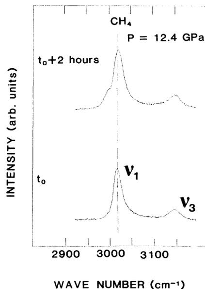
FIG. 1. Evolution with time of the  $\nu_1$  and  $\nu_3$  phonons at 12.4 GPa. The lower spectrum shows the peaks just after the pressure was increased and the upper one the same modes two hours later, showing the shift of the main peaks and the appearance of a shoulder in the low-energy side.
