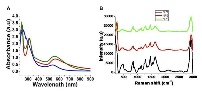
Figure 3 (A) normalized UV-Vis absorption of Gd@AuNPs: NP1 (red line), NP2 (blue line) and NP3 (green line) in the range 300–900 nm and (B) Raman spectra Gd@AuNPs (NP1-NP2-NP3) products. Experimental conditions:  $\lambda_{exc}$  = 785 nm; laser power 20 mW; accumulation time 180 s.
