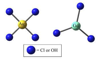
Figure 4 The square planar  $(AuX_4)^+$  precursor and the GdX<sub>3</sub> precursor with X = Cl or OH.
