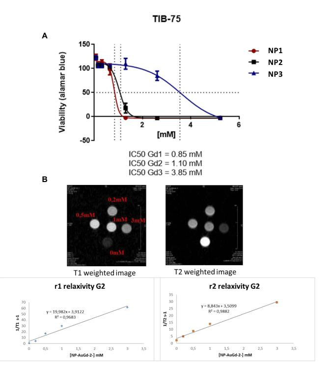
Figure 6 (A) Viability by Alamar Blue assay of TIB-75 (hepatocytes) cell lines after incubation with Gd@AuNPs (NPI-NP2-NP3); (B) Examples of MRI images of TI and T2 weighting of Gd@AuNPs recorded at 7T showing the efficient TI type features of the contrast agent for MRI at 7T with hyper signal for higher Gd concentration.
