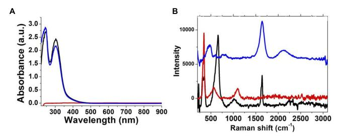
Figure I (A) UV-Vis absorption of HAuCl<sub>4</sub>  $3H_2O$  (black line), GdCl<sub>3</sub>\*6H<sub>2</sub>O (red line); Au–Gd complex (blue line) in the range 200–900 nm (B) Raman spectra of Gd@Au complex (blue line) in the range 200–3000 cm<sup>-1</sup>, compared to HAuCl<sub>4</sub>  $6H_2O$  (black line), GdCl<sub>3</sub>  $6H_2O$  (red line) as controls. Experimental conditions:  $\lambda_{exc}$  = 785 nm; laser power 20 mW; accumulation time 180 s.
