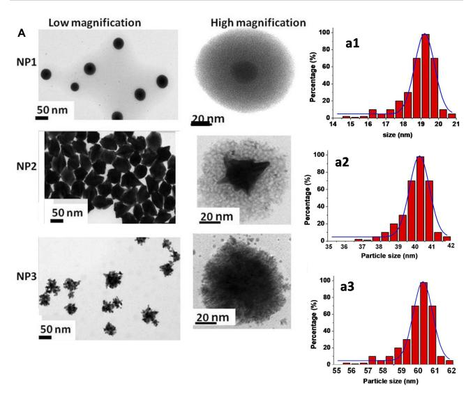
Figure 2 (A) Low and high magnification of TEM images and (a1-a2-a3) size distribution histogram of Gd@AuNPs as NP1-NP2-NP3 scale bars: 50 nm and 20 nm.
