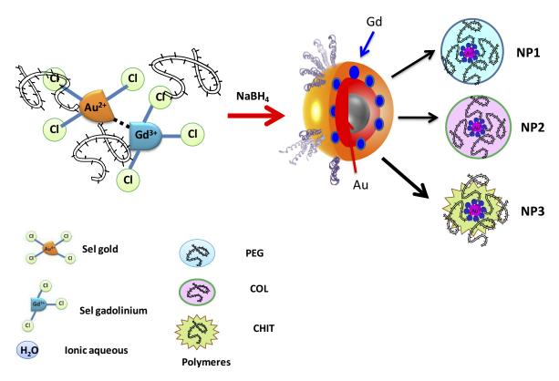
Scheme I Schematic of the proposed mechanism of  $GdCl_3$ - $AuCl_4^-$  reduction of complexation and particle formation (Gd@Au NPs) in the presence of polymer and sugar as surfactants. (Please note that drawings are not in scale and are not intended to be representative of the full sample's composition and stoichiometry.)
