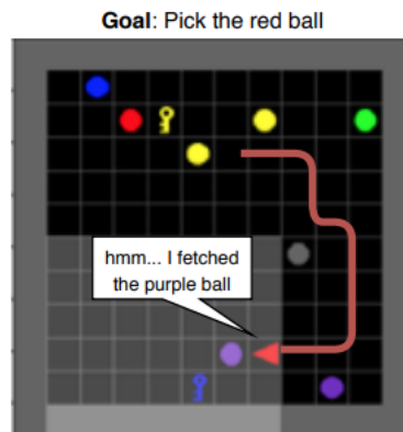
Figure 8: MiniGrid environment [74], where the agent is instructed through a textual string to pick up an object and place it next to another one. The model learns to represent the achieved goal (e.g. "Pick the purple ball") via language. As this achieved goal differs from the initial goal ("Pick the red ball"), the goal mapper relabels the episode, and both trajectories are appended to the replay buffer. Reproduced with permission of M. Seurin [28].
