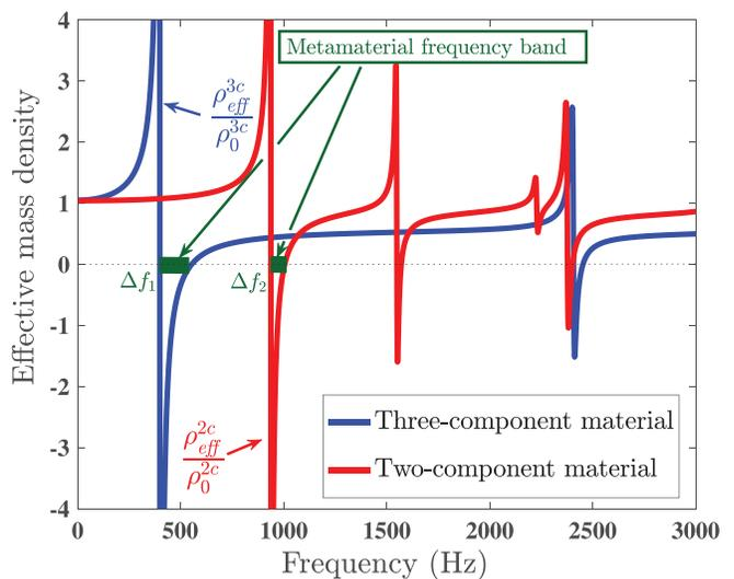
FIG. 2. (Color online) Normalized effective mass density related to two-component and three-component materials with spherical inclusions. First metamaterial bands  $\Delta f_1$  and  $\Delta f_2$ , where the effective mass densities become negative, are shown by green lines for both types of metasolids.
