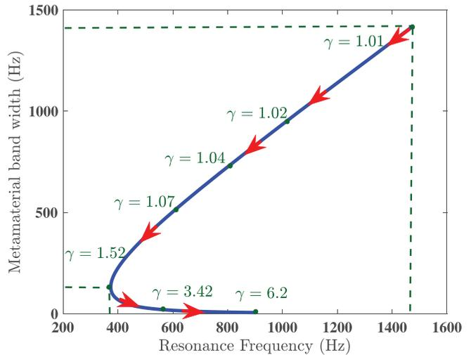
FIG. 3. (Color online) Evolution of the metamaterial bandwidth with the resonance frequency. The curve is parameterized by the form factor  $\gamma$ . The red arrows indicate the direction of increasing  $\gamma$ .
