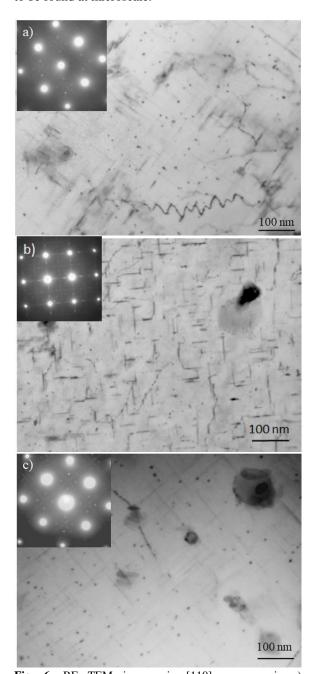
**Fig. 6.** BF TEM images in [110]<sub>Al</sub> zone axis a) L8\_180°C/8h; b) 2017A\_180°C/8h; c) L8\_ST-180°C/8h
