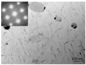
**Fig. 8.** BF-TEM images of 2017A alloy thermally aged at 180°C for 5h in [100]<sub>Al</sub> zone axis.
