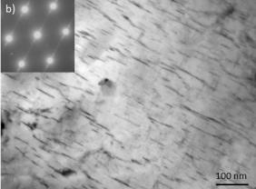
**Fig. 7.** BF-TEM images of 2017A alloy thermally aged at 100°C for 10,000h in a) [100]<sub>Al</sub> zone axis and b) in [110]<sub>Al</sub> zone axis.
