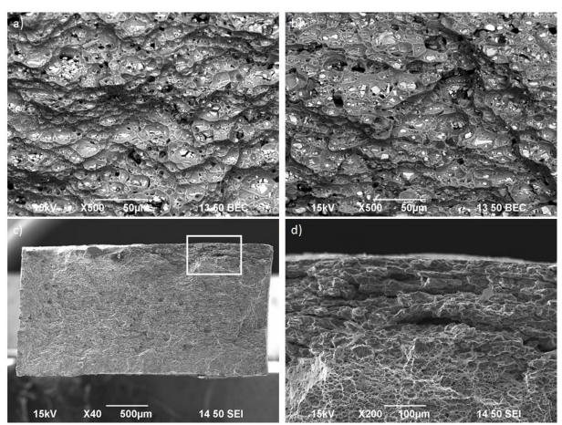
**Fig. 2.** SEM photographs of fracture surface in back-electron scattering mode for a) 2017A-AR, b) L8-AR. Images c) and d) in secondary electron mode, show fracture due to intergranular corrosion on L8-AR in the transverse direction.
