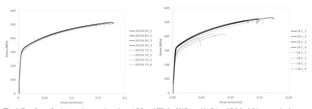
Fig. 1. True Stress/Strain curve in two orientations a) RD and TD for 2017A and b) D1 and D2 for L8 in as-received state.
