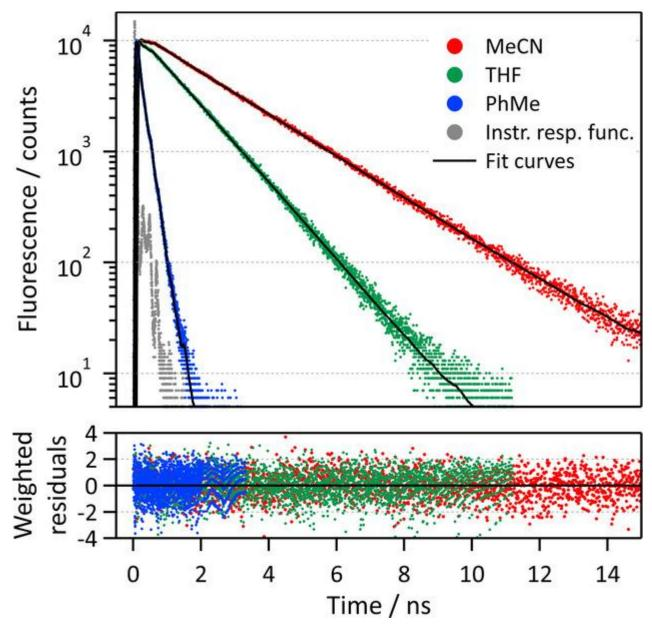
**Figure 5.** Fluorescence decay curves, instrumental response function, multiexponential fitting, and weighted residuals of (*E*)-1 in MeCN, THF, and PhMe.  $\lambda_{ex}$ =400 nm;  $\lambda_{em}$ =620 (MeCN), 590 (THF), or 550 nm (PhMe).
