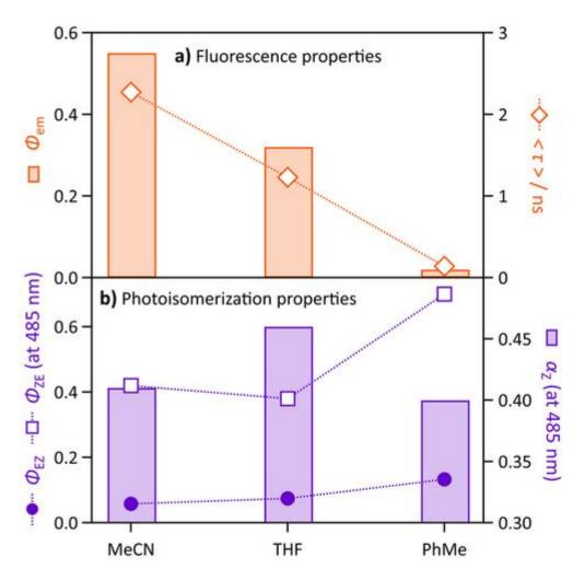
**Figure 9.** Summary of the photophysical and photochemical properties of 1 as a function of the solvent. a) Fluorescence parameters (emission quantum yield  $\Phi_{em}$ , averaged lifetime  $\langle \tau \rangle$ ) and b) photoisomerization parameters ( $E \rightarrow Z$  and  $Z \rightarrow E$  quantum yields  $\Phi_{EZ}$  and  $\Phi_{ZE}$ , respectively, and conversion yield  $\alpha_Z$  at the PSS 485 nm).  $\langle \tau \rangle$  is defined as  $\Sigma f_i \times \tau_i$ .
