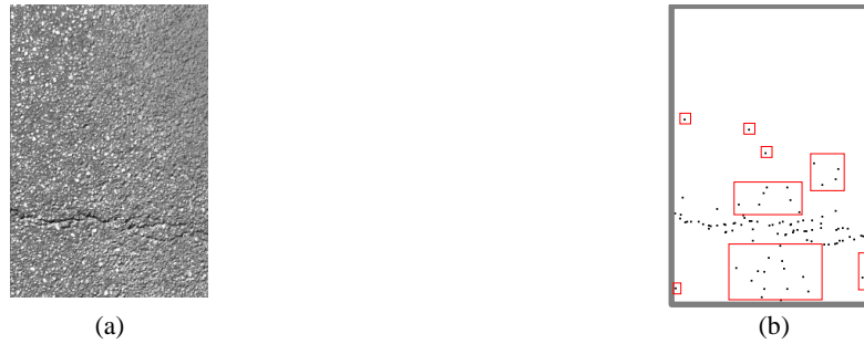
Fig. 11: (a) A gray level Aigle-RN pavement image of 311×462 pixels – (b) The selected points-of-interest (POI)
