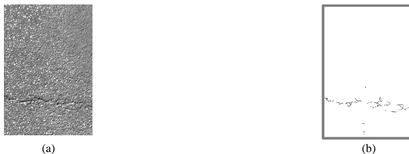
Fig. 14: (a) The original gray level pavement image shown in Fig. 11(a) – (b) The thinnest filaments obtained after applying the Dijkstra' algorithm
