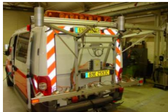
Fig. 2: Aigle-RN system installed on the vehicle
