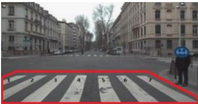
Fig. 8: Example of identified pedestrian crossing with seven strips in the original VIAPIX® image
