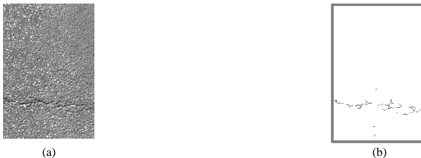
Fig. 14: (a) The original gray level pavement image shown in Fig. 11(a) – (b) The thinnest filaments obtained after applying the Dijkstra' algorithm
