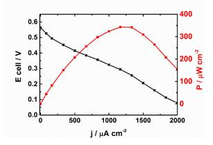
**Figure 5**: Electrochemical performances of a DEFC at 25 °C using  $Pt_{50}Rh_{50}/C$  (0.13 mg cm<sup>-2</sup>) and PdSe/C (0.13 mg cm<sup>-2</sup>) as anode and cathode catalysts, respectively; the anodic compartment contains 1 mol L<sup>-1</sup> NaOH and 1 mol L<sup>-1</sup> ethanol separated to the cathodic one by an AEM from Fumatech.
