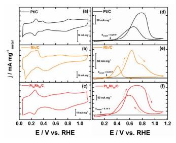
**Figure 3**: Voltammograms (CVs) of Pt and Rh based electrode materials prepared from the revisited BAE route. These CVs were recorded at room temperature and 10 mV s<sup>-1</sup> and in 1 mol L<sup>-1</sup> NaOH, in the absence (a, b and c) and the presence of 0.2 mol L<sup>-1</sup> ethanol (d, e and f).
