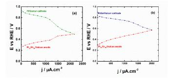
**Figure 4**: E-j polarizations curves obtained at the electrodes of a DEFC operating at room temperature and in alkaline medium. a) (-)  $Pt_{50}Rh_{50}/C / 1.0 \text{ mol } L^{-1} \text{ ethanol } // 1.0 \text{ mol } L^{-1} \text{ NaOH, } O_2 / Pt/C (+); b) (-) <math>Pt_{50}Rh_{50}/C / 1.0 \text{ mol } L^{-1} \text{ ethanol } // 1.0 \text{ mol } L^{-1} \text{ NaOH, } O_2 / PdSe/C (+)$
