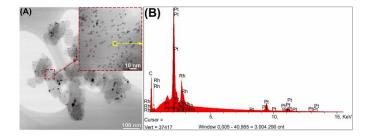
Figure 2: (a) TEM images for Pt<sub>50</sub>Rh<sub>50</sub>/C material. (b) EDX spectra of Pt<sub>50</sub>Rh<sub>50</sub>/C particle.
