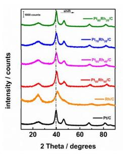
**Figure 1**: XRD patterns of the carbon supported  $Pt_xRh_y$  materials prepared from the revisited BAE method.
