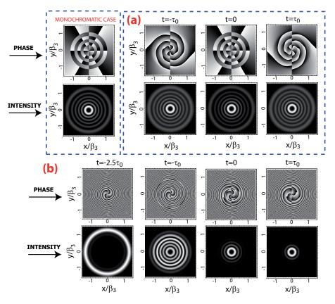
Fig. 3. Intensity and phase in Cartesian coordinates for the pulselet  $\mathscr{LG}_{5,3}$  evaluated at the snapshots indicated in the figure with (a) s = f and (b) s = 5f. It is also displayed the instantaneous intensity and phase for the monochromatic case  $\mathscr{LG}_{5,3}^{Mon}$  with s = f. Intensity graphs are normalized to its maximum value, while the gray-scale in the phase representation runs from  $-\pi$ , black, to  $+\pi$ , white, radians. Parameters are the same than in Fig. 2.
