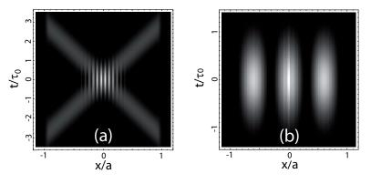
Fig. 6. Temporal evolution of the intensity as a interference of two spatial top-hat ultrafast beams with (a) a = 1.4 mm and (b)  $a = 70 \,\mu$ m, for the case s = f and  $b = \pm 1.4$  mm. The axial extents are shown in relation to the radius *a*. The parameters are the same than in Fig. 2.
