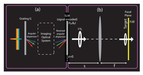
Fig. 1. (a) Approach to implement the encoded signal in phase-only computer generated holograms to the whole spectrum of the pulse. The imaging optical system cancels out the spatial chirp at the 2D SLM and makes the approach nondispersive. (b) Typical arrangement for laser micro-machining in which the spatial pulse shaping at the focus is desired.
