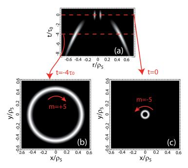
Fig. 7. (a) Temporal evolution of the intensity at the focal plane by using a signal composed by the superposition of  $LG_{0,5}$  and  $LG_{0,-5}$  modes with  $w_0 = 50$  and  $400 \,\mu$ m, respectively. Transverse intensity evaluated at the snapshots  $t = -4\tau_0$  (b) and t = 0 (c). The topological charge jumps from m = 5 to m = -5 as the pulse evolves in time.
