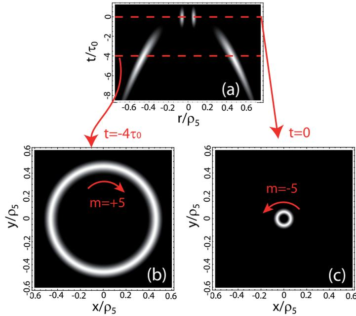
Fig. 7. (a) Temporal evolution of the intensity at the focal plane by using a signal composed by the superposition of  $LG_{0,5}$  and  $LG_{0,-5}$  modes with  $w_0 = 50$  and  $400 \mu\text{m}$ , respectively. Transverse intensity evaluated at the snapshots  $t = -4\tau_0$  (b) and  $t = 0$  (c). The topological charge jumps from  $m = 5$  to  $m = -5$  as the pulse evolves in time.
