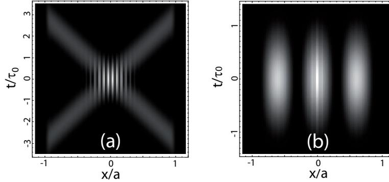
Fig. 6. Temporal evolution of the intensity as a interference of two spatial top-hat ultrafast beams with (a)  $a = 1.4$  mm and (b)  $a = 70 \mu\text{m}$ , for the case  $s = f$  and  $b = \pm 1.4$  mm. The axial extents are shown in relation to the radius  $a$ . The parameters are the same than in Fig. 2.
