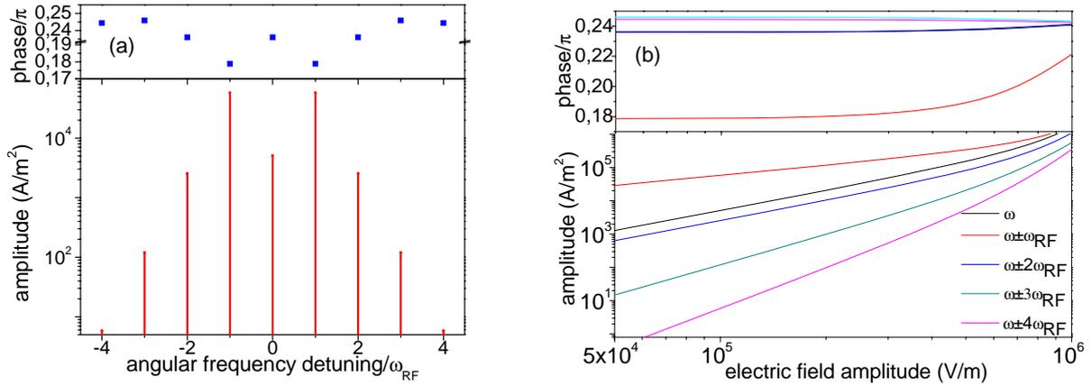
Figure 1. (a) Amplitude and phases of spectral components generated with an optical beat at  $\omega = 2\pi \times 2$  THz and a radiofrequency modulation with amplitude  $E_{RF} = 10^5$  V/m at  $\omega_{RF} = 2\pi \times 1$  MHz. The other parameters used for the calculations are taken from Table 1. (b) Dependences of amplitudes and phases in multifrequency generation in the photomixer with an alternative electric field.
