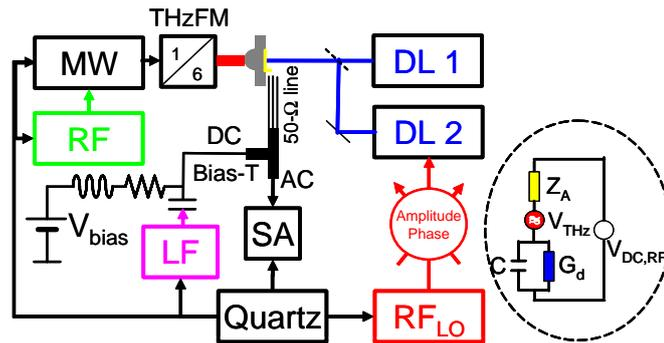
Figure 3. Experimental setup. DL1, DL2 diode lasers, SA spectrum analyzer, THzFM frequency multiplier. LF, RF, RF<sub>LO</sub>, MW synthesizers referenced to a GPS-disciplined Quartz. Inset: equivalent model for the photomixer.  $Z_A$  antenna impedance,  $C$  electrodes capacitance,  $G_d$  optically-driven nonlinear photoconductance,  $V_{\text{THz}}$  antenna-induced Thévenin voltage,  $V_{\text{DC,RF}}$  alternative voltage superposed on a continuous voltage.
