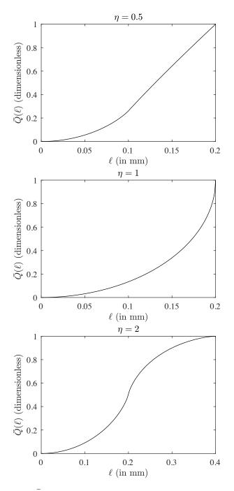
Figure 4: Normalized CLD  $\overline{Q}$  associated to a Dirac distribution of spheroids at r = 1mm for  $\eta = 0.5, 1, 2$ .
