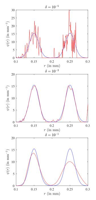
Figure 5: Estimation of the PSD by the Tikhonov regularization method. In blue: the PSD given by (24). In red: the PSD estimated by the Tikhonov regularization method for  $\delta = 10^{-5}$ ,  $10^{-3}$ ,  $10^{-1}$ .
