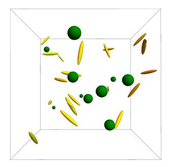
Figure 6: Simulated suspension of ideal particles of two shapes, distributed in size: spheres  $(\eta = 1, \text{ in green})$  and prolate spheroids  $(\eta = 6, \text{ in yellow})$ , in a cubic volume of 1cm<sup>3</sup>.
