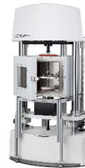
Tensile test on a BOSE Electroforce 3230 machine. Cross head speed 0.01 \text{ mm}\cdot\text{s}^{-1} . Strain measure with grips displacement. Load cell of 20N.
