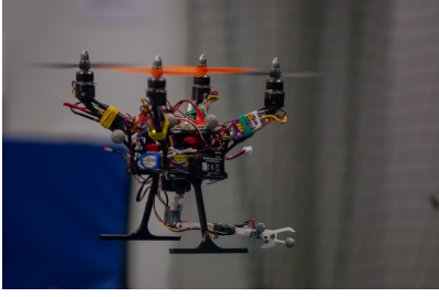
Fig. 3: Mini-quadcopter with its manipulator arm in flight.
