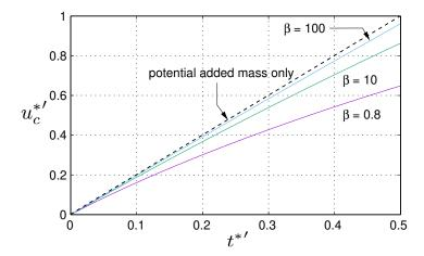
FIGURE 16. Variation of the rescaled velocity with rescaled time at  $Re^* = 200$  for different mass ratios, showing the collapse of the curves for small times.
