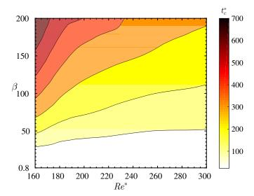
FIGURE 17. Characteristic time  $t_c^*$  for the onset of vortex shedding, as function of Reynolds number and density ratio.
