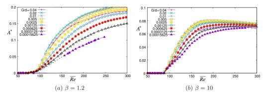
FIGURE 13. Amplitude  $A^*$  of velocity oscillations (scaled by the mean velocity).
