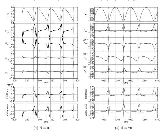
FIGURE 25. Time histories of the oscillation amplitude and force components for  $Re^* = 250$  and two density ratios. From top to bottom, the subfigures show:  $X^*$  – cylinder displacement with respect to the motion at constant mean velocity;  $F_{x,p}$  – pressure force coefficient without added mass;  $F_{am}$  – added mass force coefficient;  $F_{x,\nu}$  – viscous force coefficient;  $F_T$  – force coefficient from torque; total force coefficient; and vortex force coefficient.
