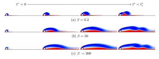
FIGURE 18. Initial development of the flow (vorticity contours) up to the shedding of the first vortex at time  $t_c^*$ , for  $Re^* = 160$  and different density ratios.
