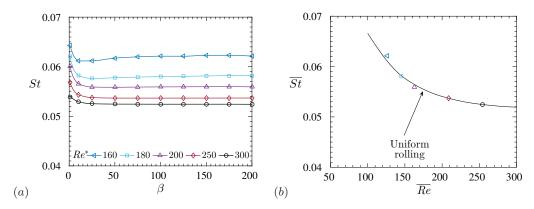
FIGURE 23. (a) Strouhal number as function of density ratio for different Reynolds numbers. For  $\beta \geq 50$ , the Strouhal number is practically constant. Its mean value  $\overline{St}$  in this range is shown as function of  $\overline{Re}$  in (b) and compared to the uniform-rolling case.
