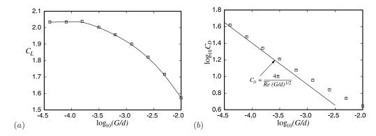
FIGURE 3. Variation of (a) lift coefficient and (b) drag coefficient with gap size. The prediction from lubrication theory in the limit of vanishing gap size is shown by the solid line in (b).  $\overline{Re} = 50$ .
