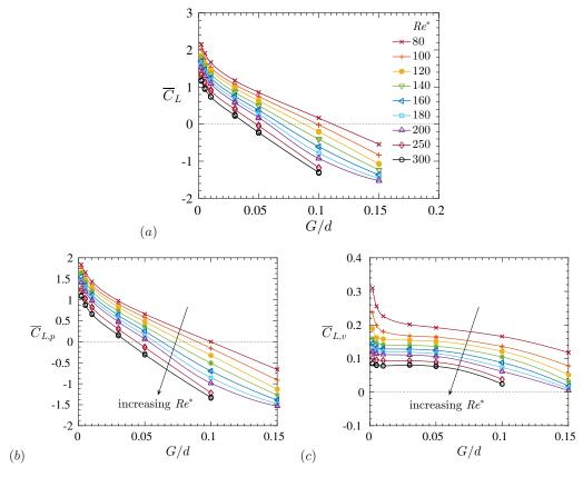
FIGURE 10. (a) Mean lift coefficient  $\overline{C}_L$  as a function of the gap size G/d for  $Re^* = 80$ –300. (b,c) Pressure and viscous components of the lift force.
