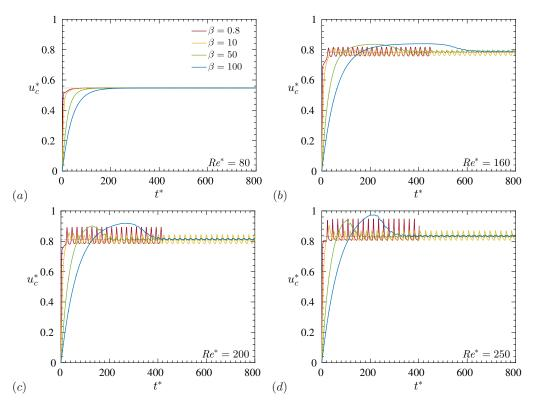
FIGURE 15. Temporal evolution of the cylinder velocity for different Reynolds numbers and density ratios.
