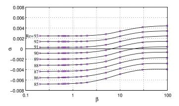
FIGURE 6. Non-dimensional growth rate  $\sigma$  (scaled by  $u_c/d$ ) of the most unstable periodic mode as a function of density ratio  $\beta$  for different Reynolds numbers.
