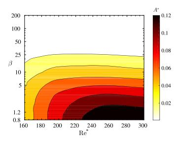
FIGURE 20. Amplitude  $A^*$  of cylinder velocity oscillations (scaled by the mean velocity), as function of Reynolds number and density ratio.
