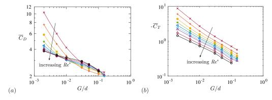
FIGURE 12. Mean (a) drag coefficient and (b) torque coefficient for  $Re^* \ge 80$  (see legend in figure 10a).
