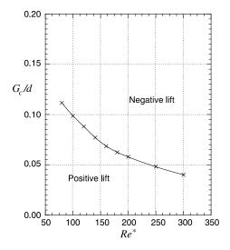
FIGURE 11. Relationship between Reynolds number and critical gap height for the change of sign of the lift force.
