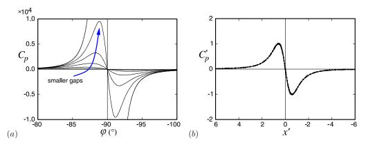
FIGURE 2. (a) Pressure coefficient distribution in the vicinity of the gap for different gap sizes:  $G/d = 0.005/2^n$ , n = 0,...,4. (b) Rescaled distribution based on lubrication theory (see text for details).  $\overline{Re} = 50$ .
