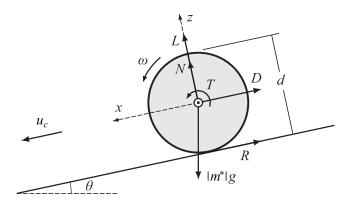
FIGURE 1. Schematic of a cylinder rolling along an inclined plane of slope angle  $\theta$ . Its translational and angular velocities are  $u_c$  and  $\omega$ , respectively. The frame of reference (x, z) is attached to the centre of the body, and the different forces exerted on it are illustrated: the fluid forces (drag D, lift L and torque T), the mechanical forces (reactions of the wall on the body, N and R) and gravity/buoyancy ( $|m^*|g$ ).
