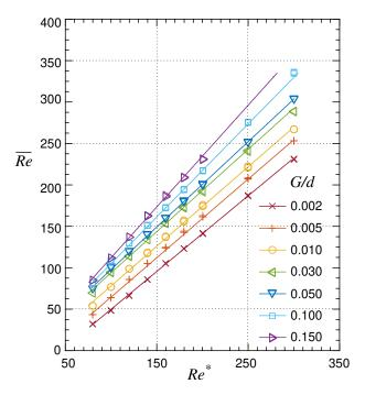
FIGURE 9. Relationship between the Reynolds number  $\overline{Re}$  based on the asymptotic (mean) velocity and the modified Reynolds number  $Re^*$ . The different curves correspond to different gap ratios.
