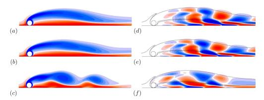
FIGURE 8. Vorticity fields for the steady rolling cylinder. Left column: (a) steady solution at Re = 90; (b, c) saturated unsteady flow at Re = 89.4 and Re = 90, respectively. Right column: (d) dominant linear instability mode of the steady flow at Re = 90; (e, f) perturbation at saturation for Re = 89.4 and Re = 90; respectively. The lines are contours of the steady vorticity field for  $\omega_z = \pm 0.1 U/d$ .
