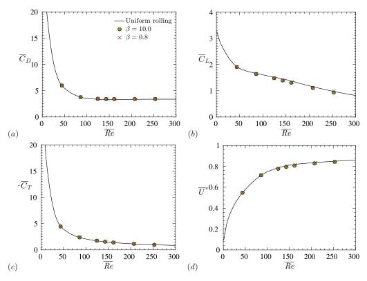
FIGURE 24. Mean (a) drag, (b) lift and (c) torque coefficients. The lines show the results for uniform rolling. (d) Asymptotic mean velocity. The line represents the prediction in equation (2.18).
