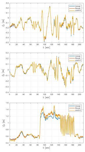
Fig. 2. Camera positions given by the proposed Riccati observer, *solvePnP()* algorithm and MOCAP ground truth.
