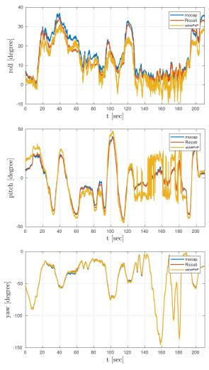
Fig. 3. Camera attitudes (Euler angles) given by the proposed Riccati observer, solvePnP() algorithm and MOCAP ground truth.
