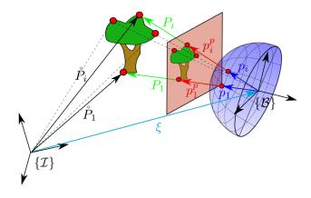
Fig. 1. Intuitive representation of inertial coordinates  $\mathring{P}_i$ , planar projective coordinates  $p_i^p$  and spherical projective coordinates  $p_i$  of the  $i^{\mathrm{th}}$  source point.
