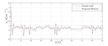
Fig. 6. Estimated and ground-truth depth inverse  $(m^{-1})$  versus time (s)
