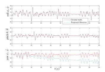
Fig. 4. Estimated and ground-truth attitudes represented by roll, pitch and yaw Euler angles (deg) versus time (s)
